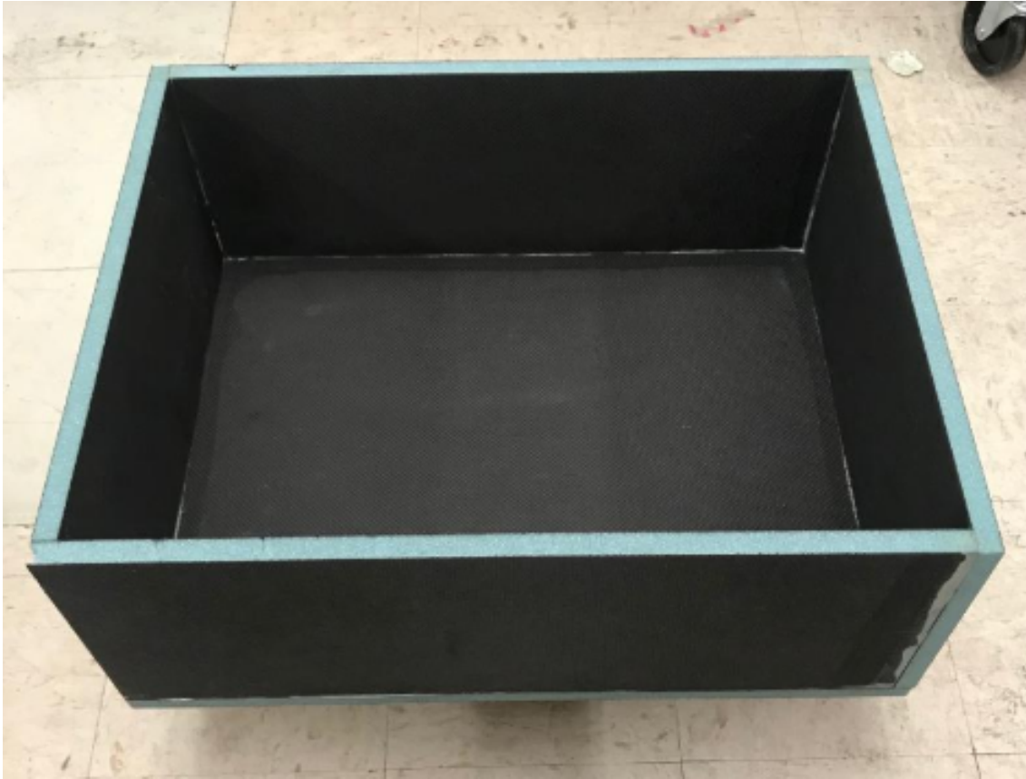
Figure 3.8: CFRP Box Freshly Assembled with Epoxy
