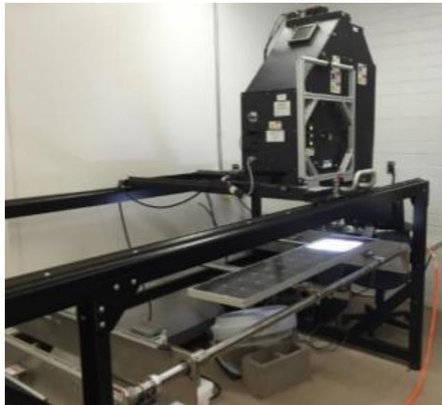
Figure 3.8: Solar simulator for indoor IV measurements
