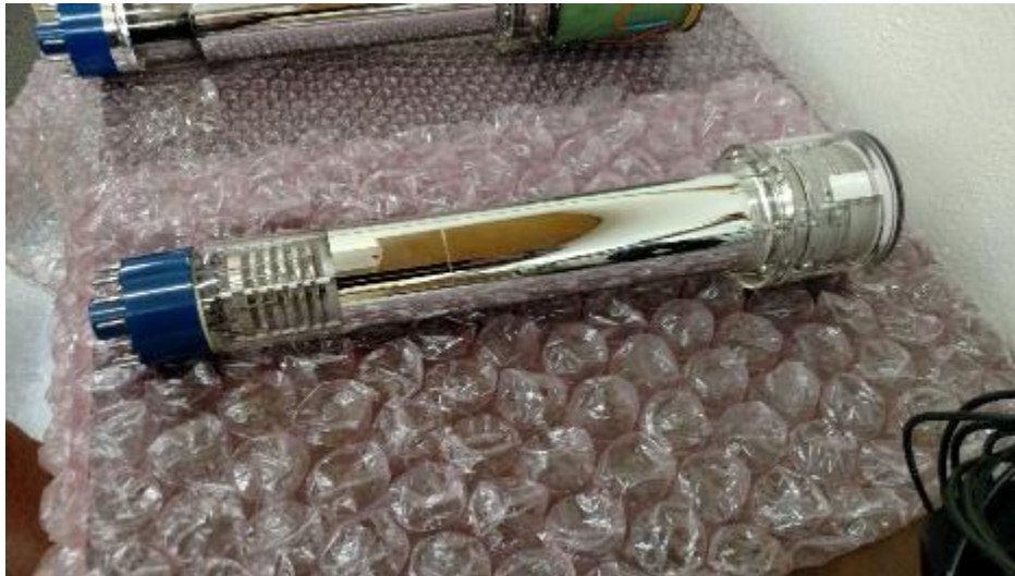
Figure 2.7. Image orthicon (photo). GE-produced image orthicon tube used at Kitt Peak Observatory by William Livingston. 87
