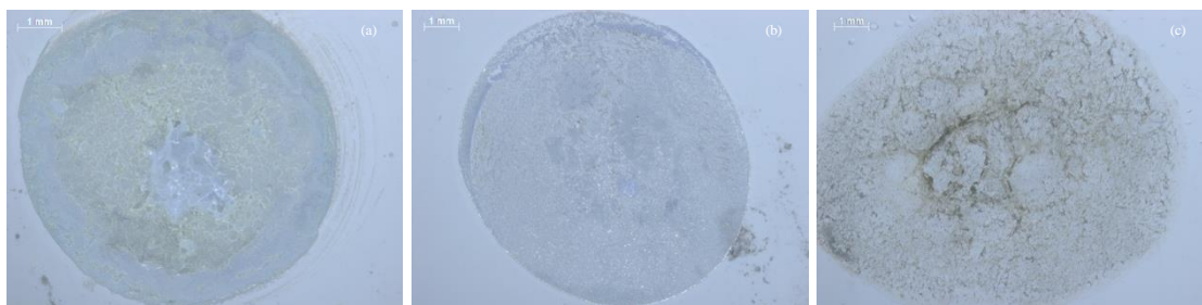
Figure 5. Dried droplets of ink pipetted onto untreated glass. Formulation was 0.1 M nickel acetate and 2 M hydrazine in a 20/80 vol % mixture of ammonia solution and polyol. Solvent and deposition temperatures are: (a) ethylene glycol, 100 °C; (b) propylene glycol, 100 °C; (c) glycerol, 150 °C.
