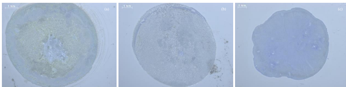
Figure 3. Common products of nickel reactive inks containing nickel acetate, hydrazine, ammonia, water, and simple alcohol or amine-based solvents. (a) green salt; (b) porous white material; (c) purple salt.
