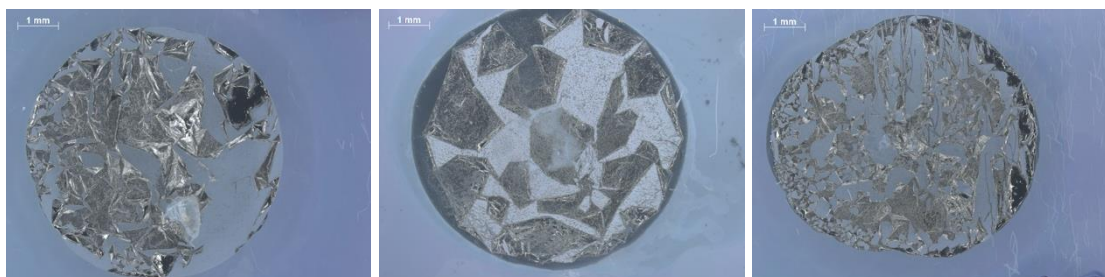
Figure 32. Deposits produced by pipetting inks (0.05 M [\text{Ni}^{2+}] , 1.84 M [\text{N}_2\text{H}_4] and 0.4 M [\text{TMAH}] in a 20/30/50 vol % mix of DI water, primary solvent, and PG respectively) onto a gold-coated glass slide at 100 °C. The primary solvent is labeled in the image.
