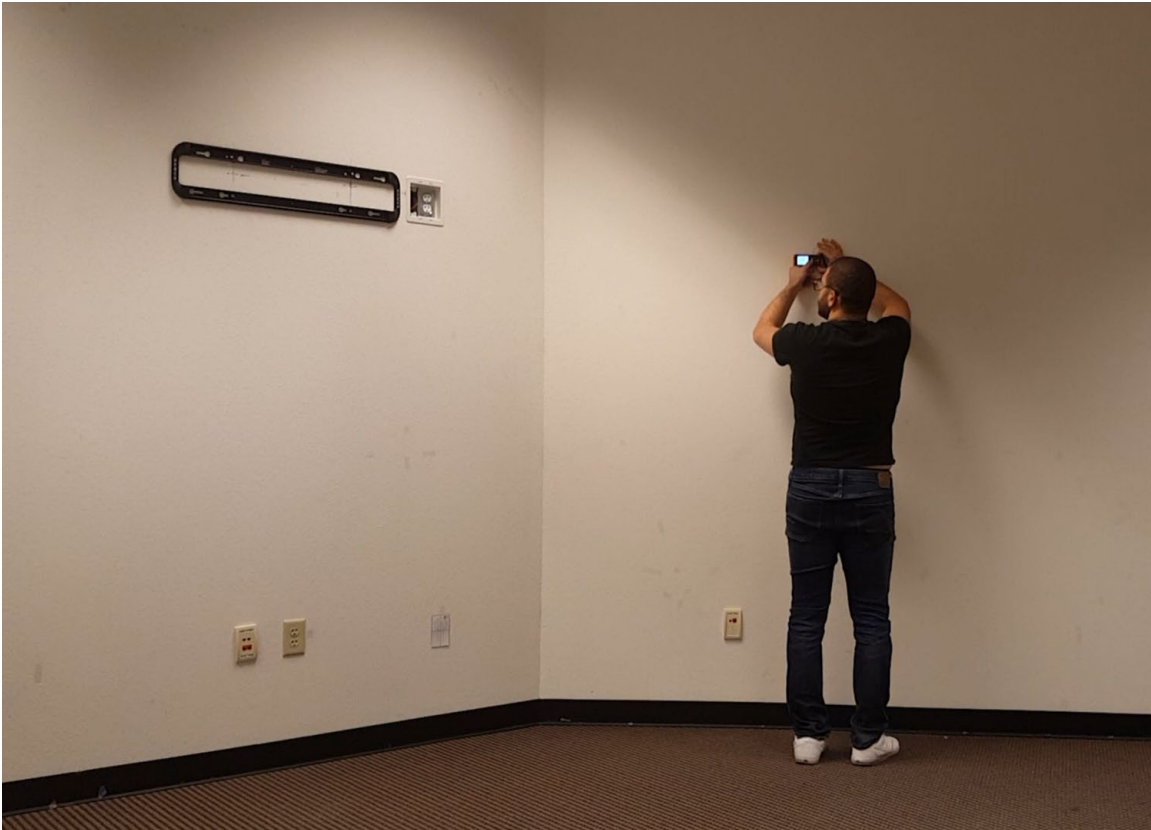
Figure 22: Researchers Measuring Point Offsets of Points Laid Out
