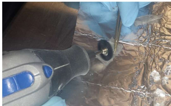
Figure 9: Plastic brush cleaning tool for cleaning the extracted EVA
