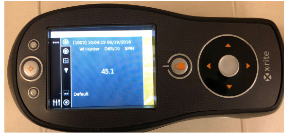
Figure 12: Colorimetry device for measuring the yellowness index
