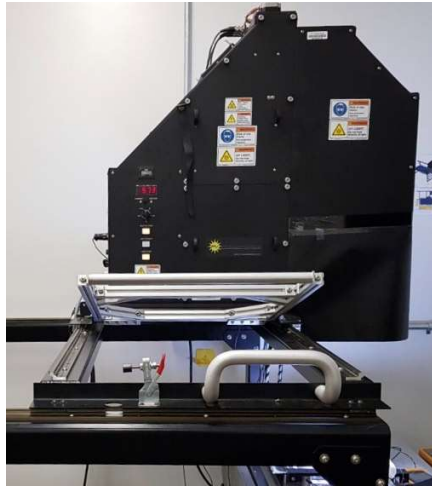
Figure 11: Experimental setup of a solar simulator for I-V measurements
