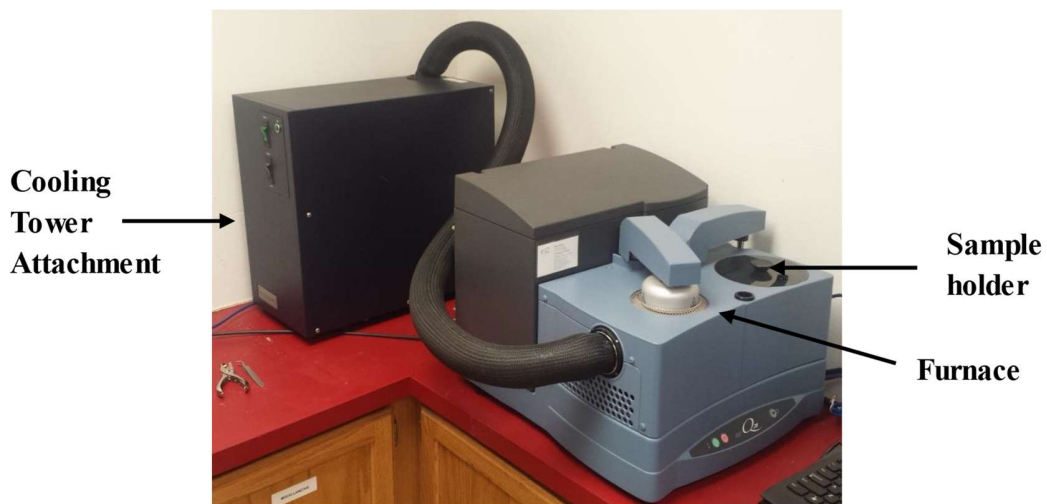
Figure 13: DSC instrument equipped with the cooling tower attachment
