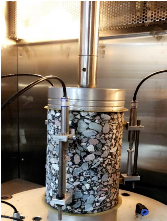
Figure 16. Instrumented dynamic modulus |E^*| test sample
