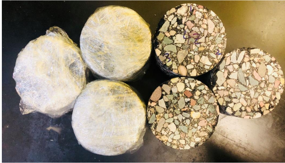
Figure 18. Dry and conditioned subsets for TSR
