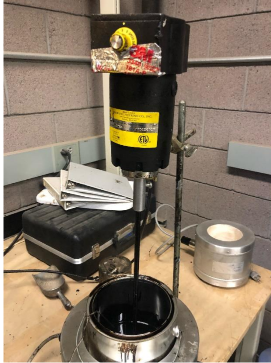
Figure 9. Blender used for preparing crumb rubber modified binder
