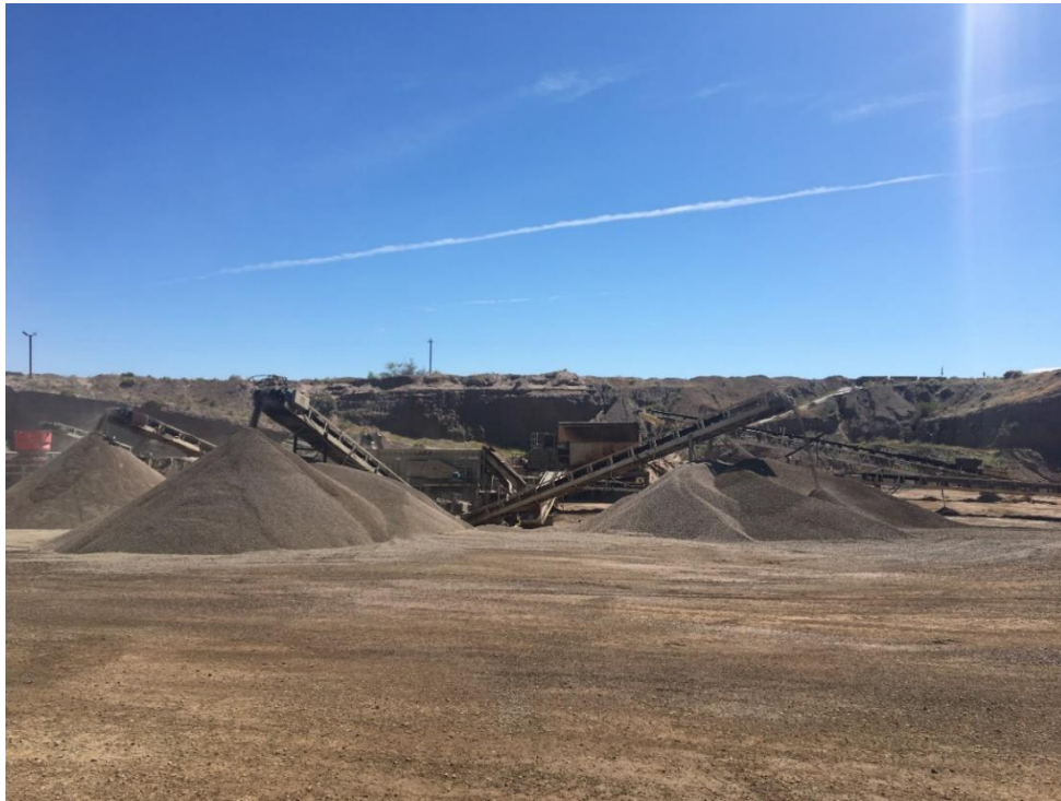
Figure 6. Aggregate stockpiles in southwest asphalt el mirage pit
