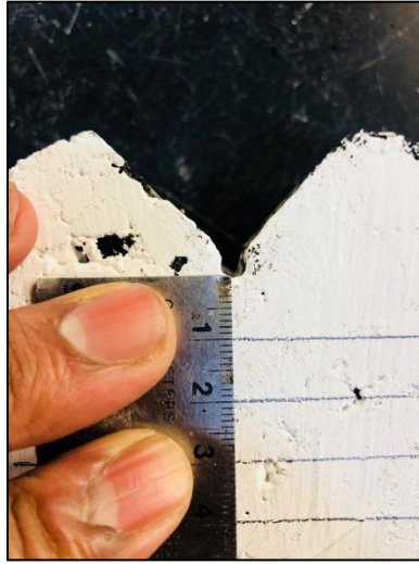
Figure 51. Close view of C* notch and crack propagation lines
