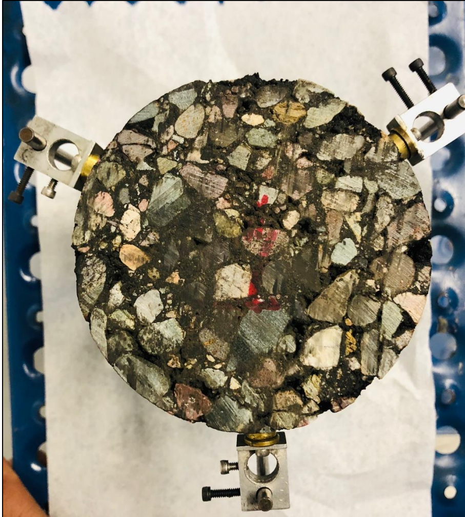
Figure 41. Dynamic modulus sample LVDT instrumentation 120° apart
