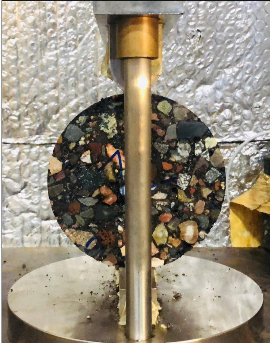
Figure 48. TSR sample testing setup
