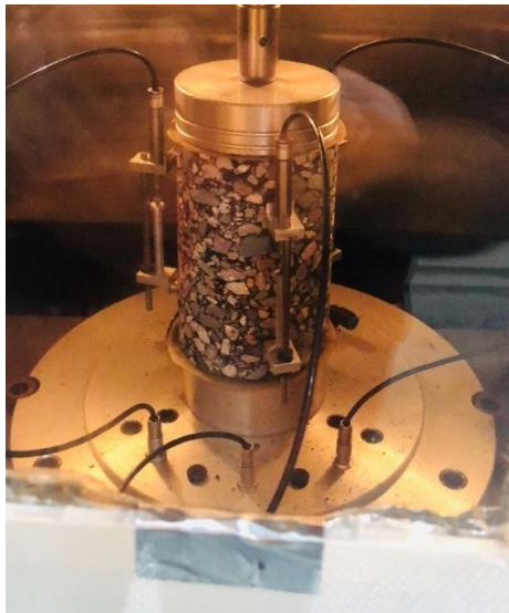
Figure 17. Set-up specimen for flow number test
