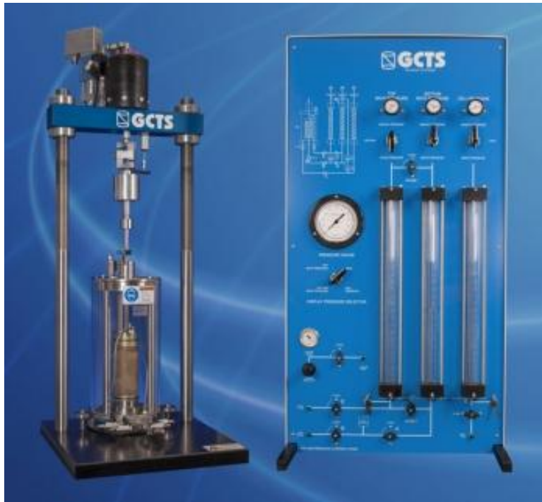
Figure 9: The STX-050 Pneumatic Soil Triaxial System (GCTS Testing Systems)
