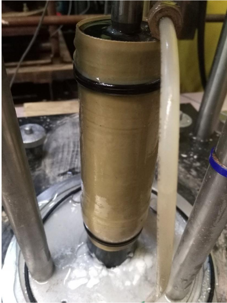
Figure 23: The ASU soil specimen after cyclic triaxial loading
