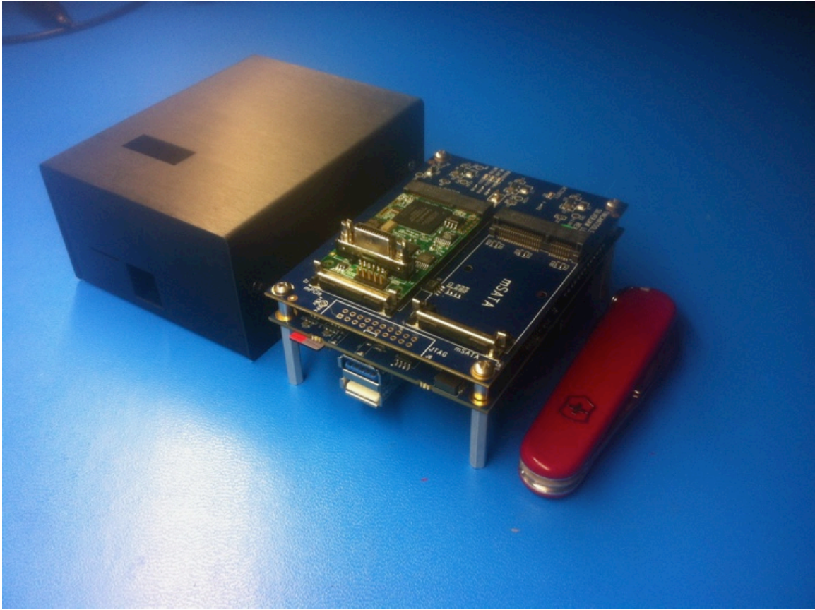
Figure 70. The instrument computer case sitting next to the instrument computer showing corresponding holes for harness connections.
