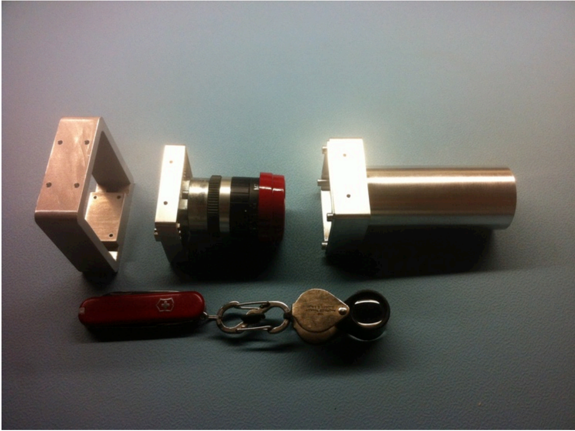
Figure 99. Exploded view of the visible camera. From left to right, a bracket designed by the spacecraft team was constructed from the spacecraft team's CAD file. The camera backplate housing holds the visible camera core and the lens was attached. For now, the red lens cap protects the lens. The frontplate and solar shade are one integrated component.
