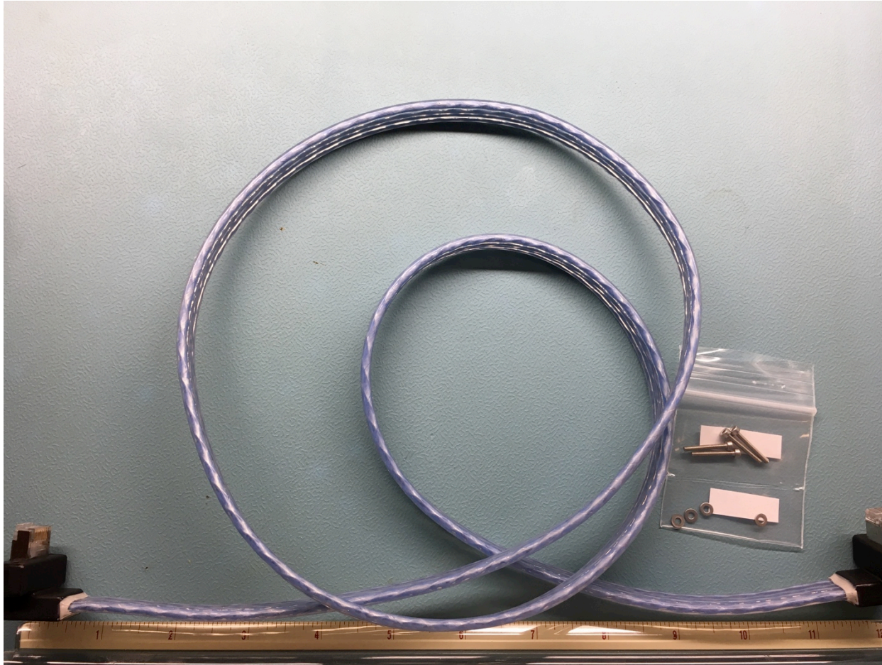
Figure 145. Ethernet Harness. The total length of the Ethernet harness was 48". There was a combined total of about 0.5" of non-usable length from the midpoint of the connector to the edge of the harness.
