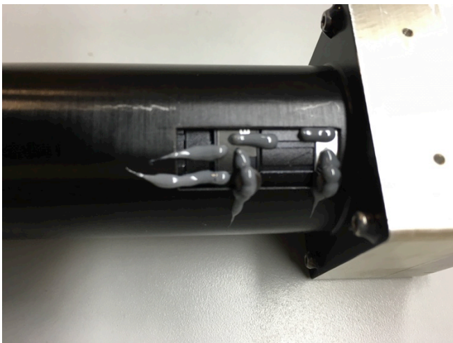
Figure 97. The lens focusing ring, aperture ring, and locking screws are staked to prevent alteration during launch. The assembly screws are also staked in the four corners of the housing.
