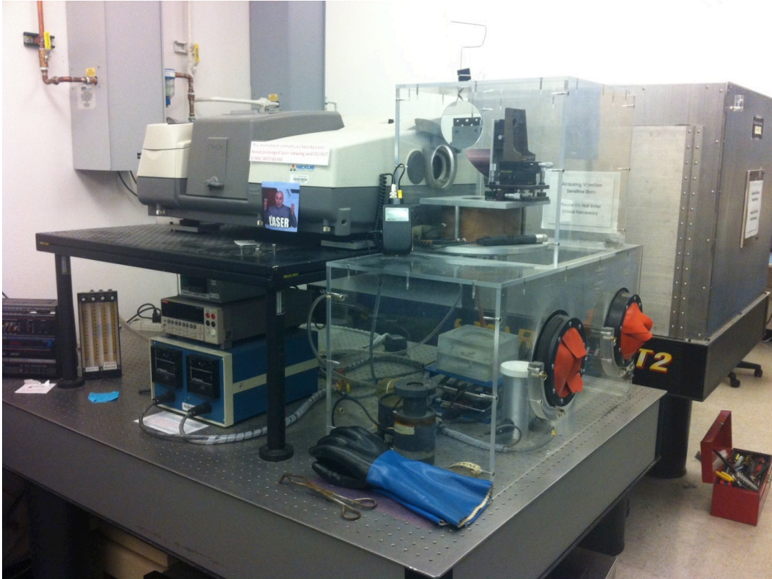
Figure 15. A) ASU Thermal Emission Spectroscopy Lab's Nicolet 670 interferometric spectrometer.
