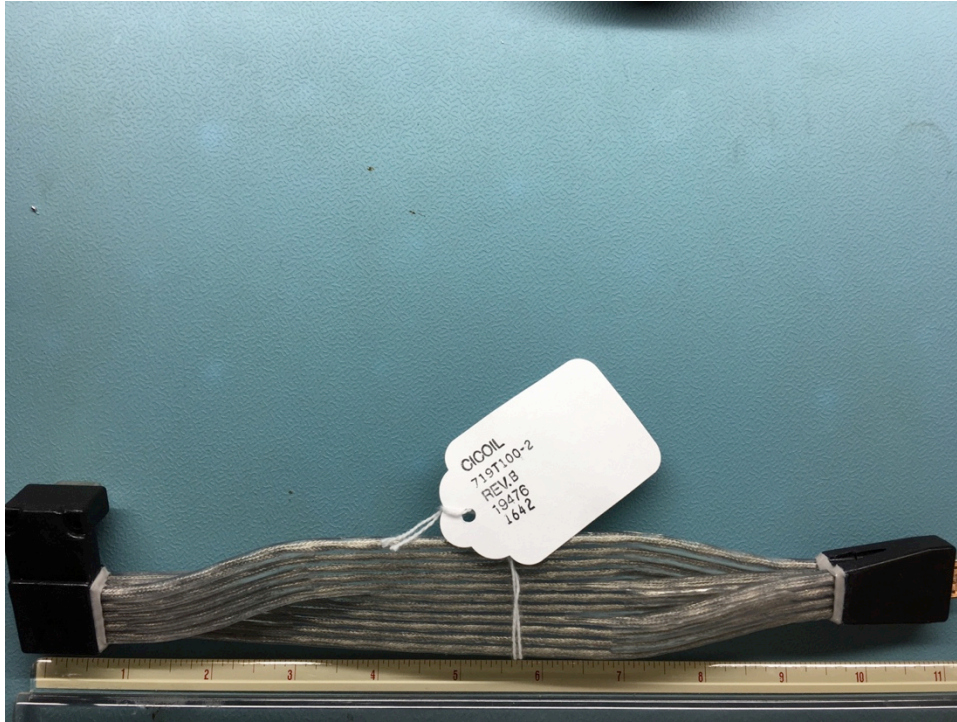
Figure 142. The Camera Link cable was 11" long. Jack screws are not shown in this image, but they have been integrated with the EM flight-like test harness and work. The distance from the center of the 90 degree bend to the edge of the harness was closer to 10.5".
