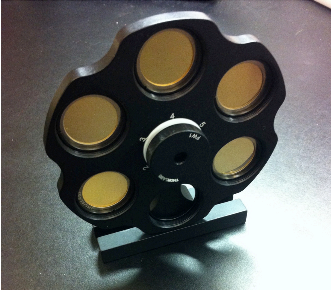
Figure 22. Gold THz band-pass filters in filter wheel. As a practical concern, extreme caution was necessary with the filters.
