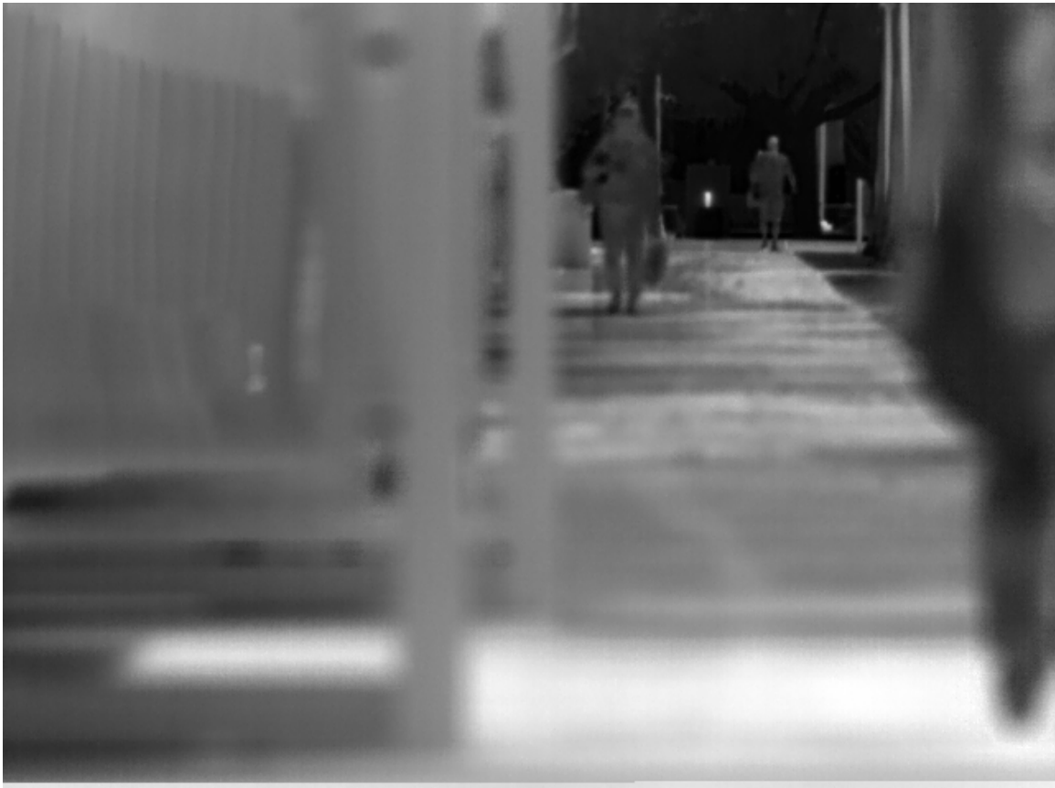
Figure 154. Infrared resolution test image of the CubeSat at 200 meters.
