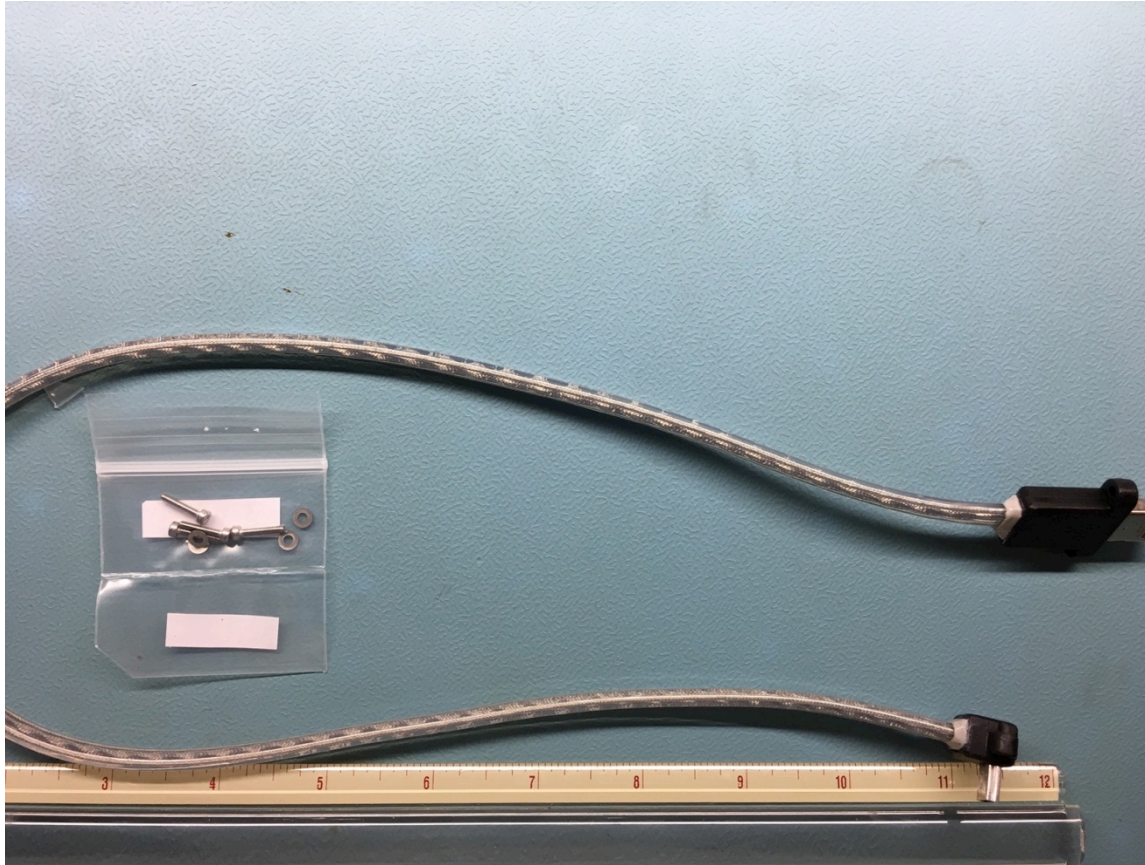
Figure 144. The visible camera data harness was about 24” from the tip of the USB to the tip of the USB mini. The effective length from the non-inserted point of the USB to the mid point of the extruded insert on the USB mini was about 23.5”.
