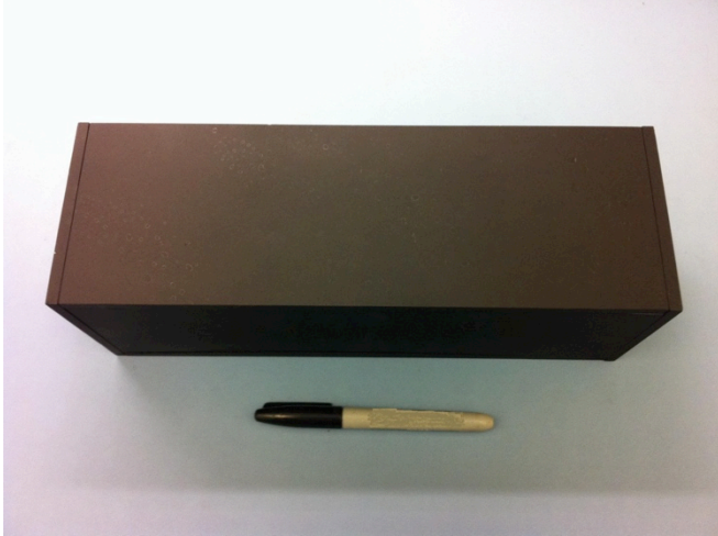
Figure 52. The sample blackbox CubeSat. (10 x 10 x 30 cm).
