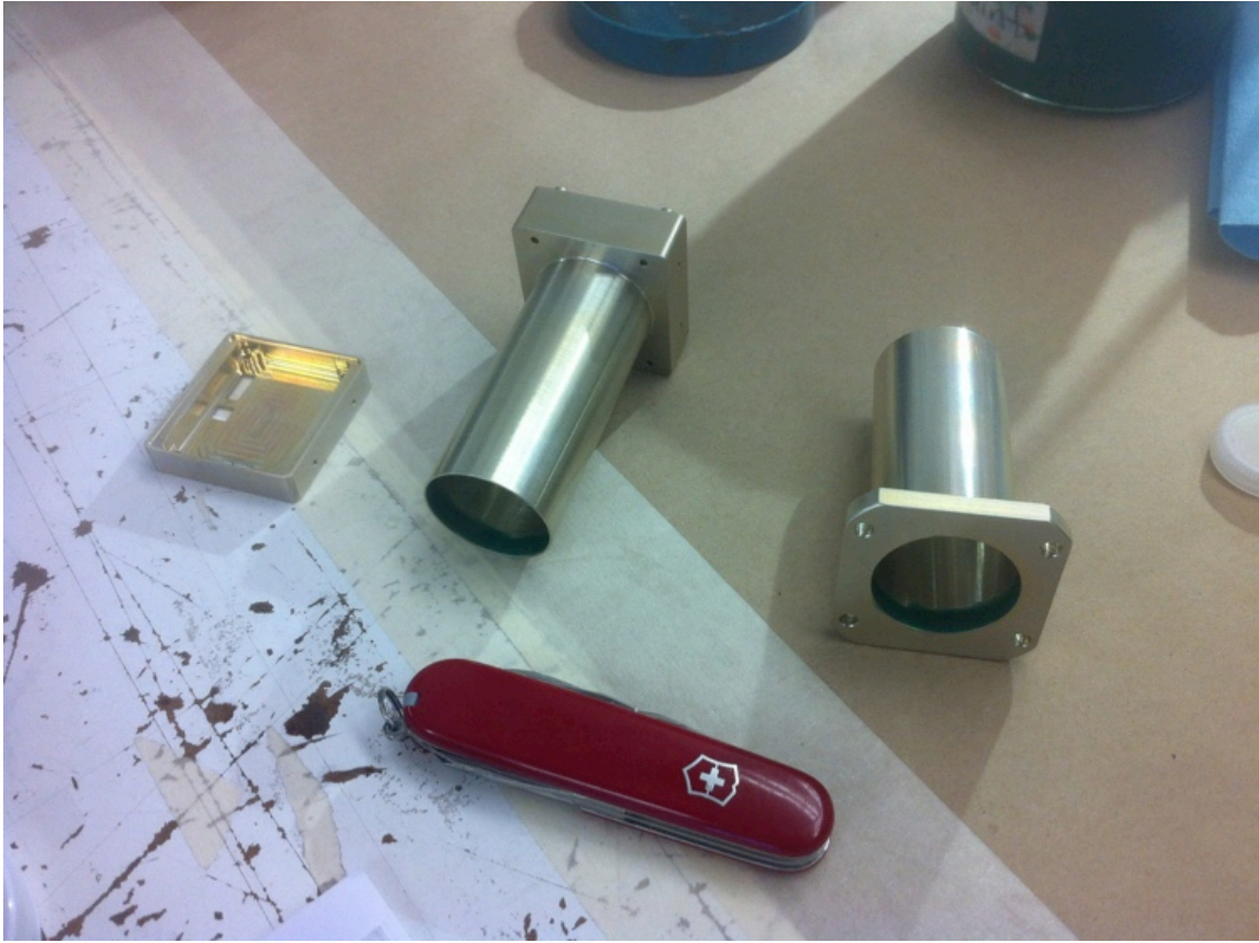
Figure 72. Visible camera parts after alodine treatment. Green masking compound was applied to protect surfaces that will not be anodized.
