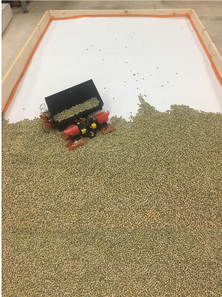
Figure 6.1: Sloped experimental test bed filled with granular media for excavation.
