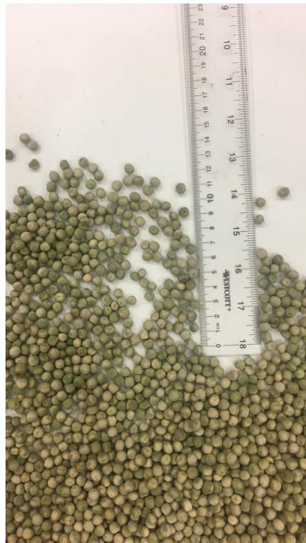
Figure 7.2: Dried peas were ultimately selected for excavation materials due to their low cost, low density and uniformly spherical shape.
