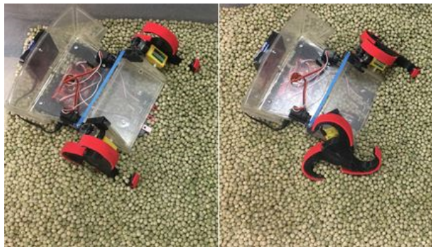
Figure 8.9: The locomoting (left) and excavating (right) modes of the first prototype
