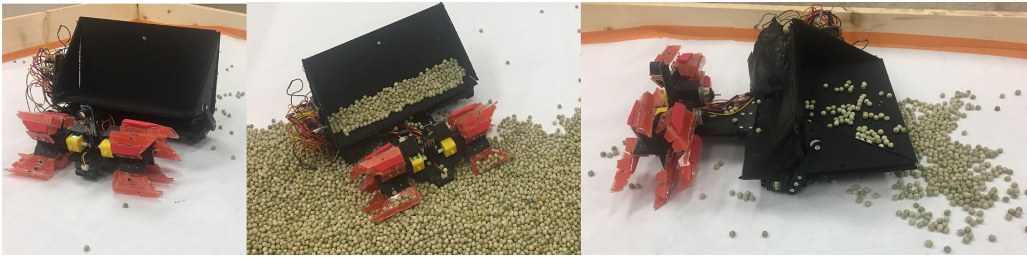
Figure 9.1: The robot in position for (1) Roaming (2) Excavating (3) Depositing
