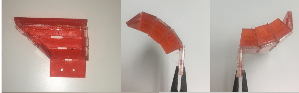
Figure 8.13: Final acrylic whogs with reinforcing fabric flex layer. Locomoting mode (center) and excavating mode (right). Rotations are limited by the whog material thickness during excavation.
