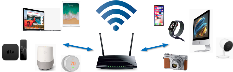
Figure 1.1: A scenario where FD TWRs are spectrally efficient - in the IoT era where huge number of devices simultaneously access a router, spectrally efficient architecture becomes more and more crucial. TWRs provide pair-wise two-way communication for devices while FD makes the router efficient.
