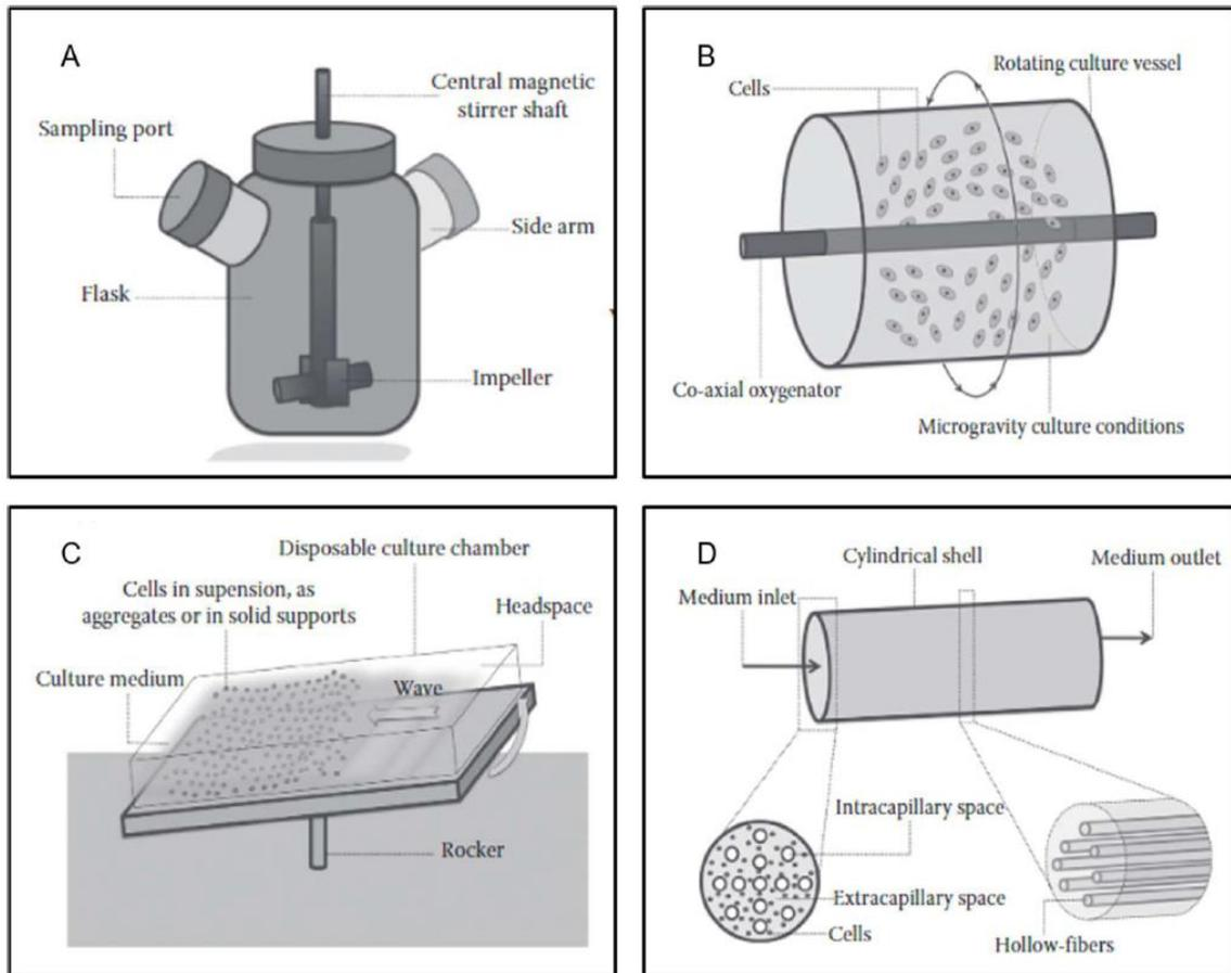
**Figure 1-3: Possible Bioreactor Configurations.** (A) Spinner flask (B) Rotating wall vessel bioreactor (C) Wave bioreactor (D) Hollow fiber bioreactor (Schaffer et al.)
