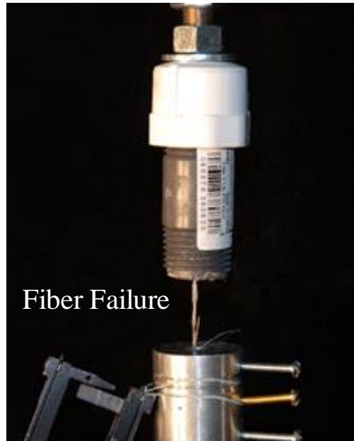
Figure 30: 35 kGy sample illustrating fiber failure before matrix failure.
