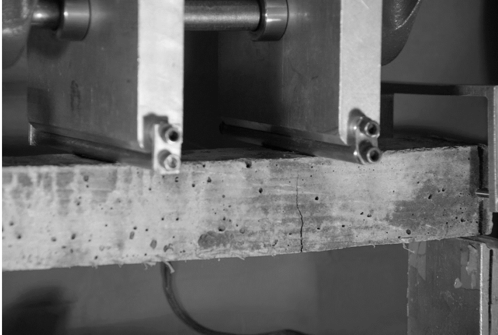
Figure 38: FRC beam specimen after testing.
