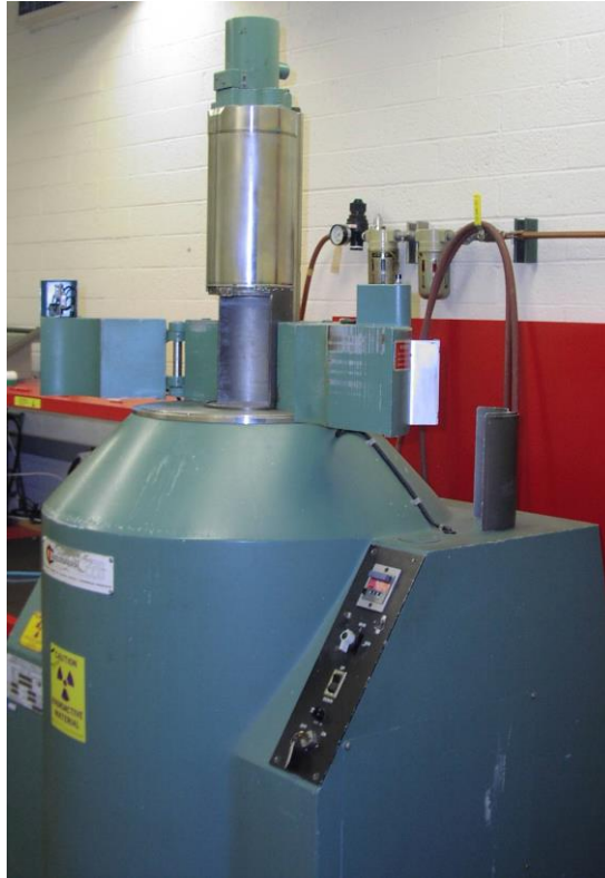
Figure 4: Gamma Cell 220 Self-Shielded irradiator with Co-60.
