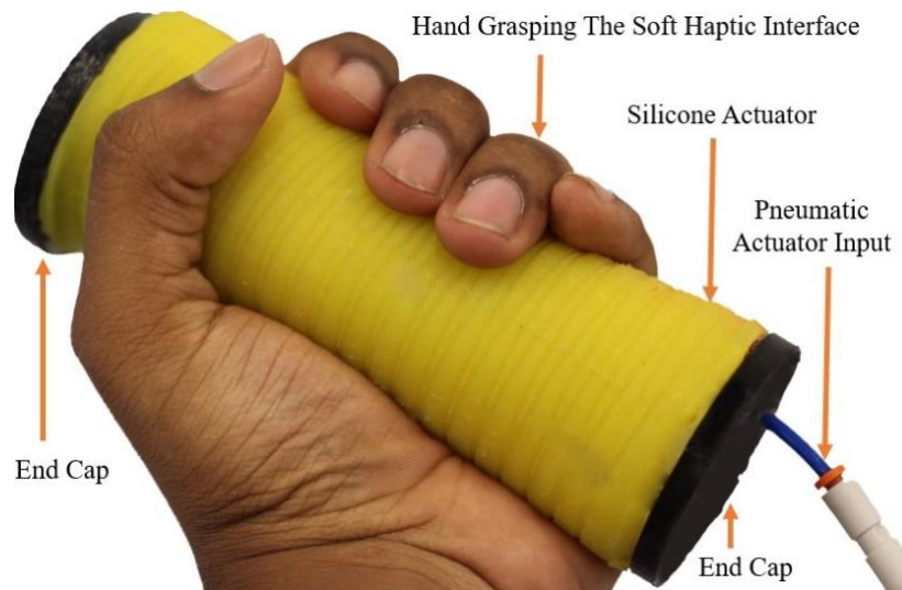
Figure 19: The prototyped soft haptic variable stiffness interface with a hand grasping it
