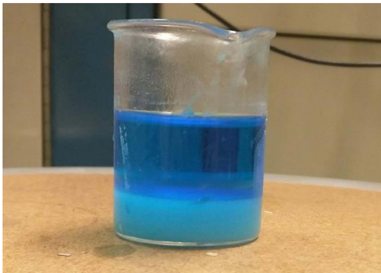
Fig. 5.5 The \text{HNO}_3 leaching solution after dissolution of four metals, Ag, Pb, Sn and Cu.
