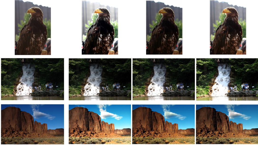
Figure 4.4: The Left Column Always Contains an Original Low-quality Image. Row 1 and 3: Columns 2, 3 and 4 Contain Images Enhanced by k nn, Picasa, and GP. Row 2: The Right Three Columns Contain Enhanced Versions Generated by GP. Please Read Text for Details 3 ©2017 IEEE.
