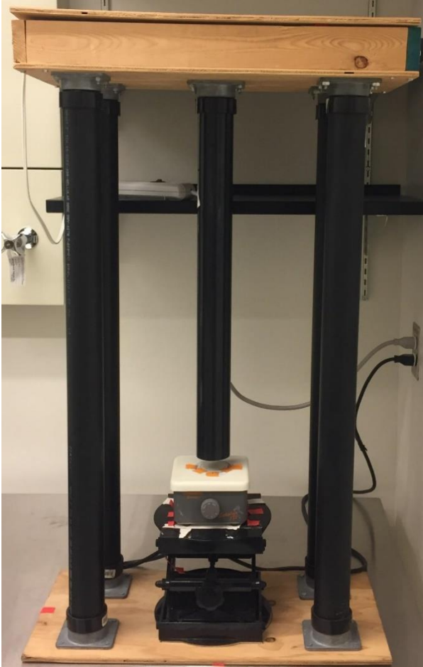
Figure 2. Picture of the Collimated Beam Apparatus Used in this Study
