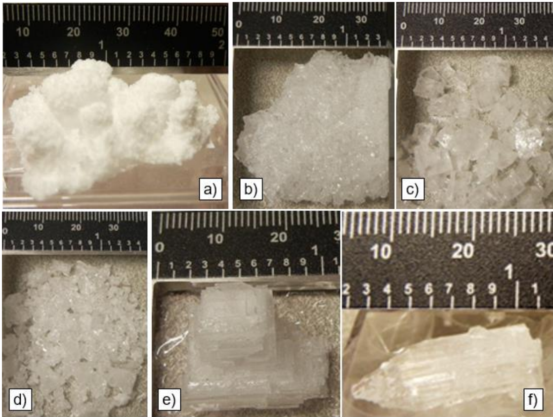
Figure 4.6. Synthetic samples used for spectral analysis. All samples are composed of halite. a) Efflorescent Crust, b) Aggregate, c) Small Cubes, d) Particles >180\ \mu\text{m} , e) Pyramid, and f) Large Crystal.
