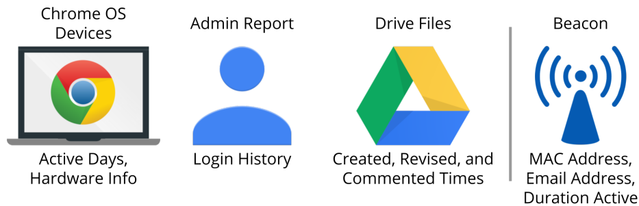
Figure 5.3: The four APIs used and the information they provide. The first three belong to G Suite and the fourth comes from Chrome.
