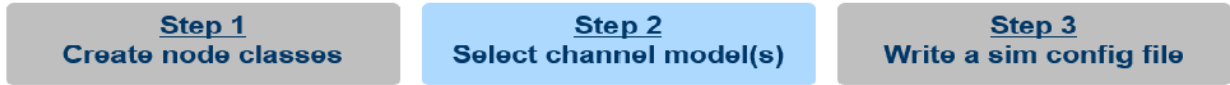
Figure 3. Steps involved in building a WiscaPDK simulation. First node class is created for a specific radio which the user wants to simulate which is then followed by selection of channel model and then the software writes a simulation configuration file which is used by WiscaComm to set the simulation in action.
