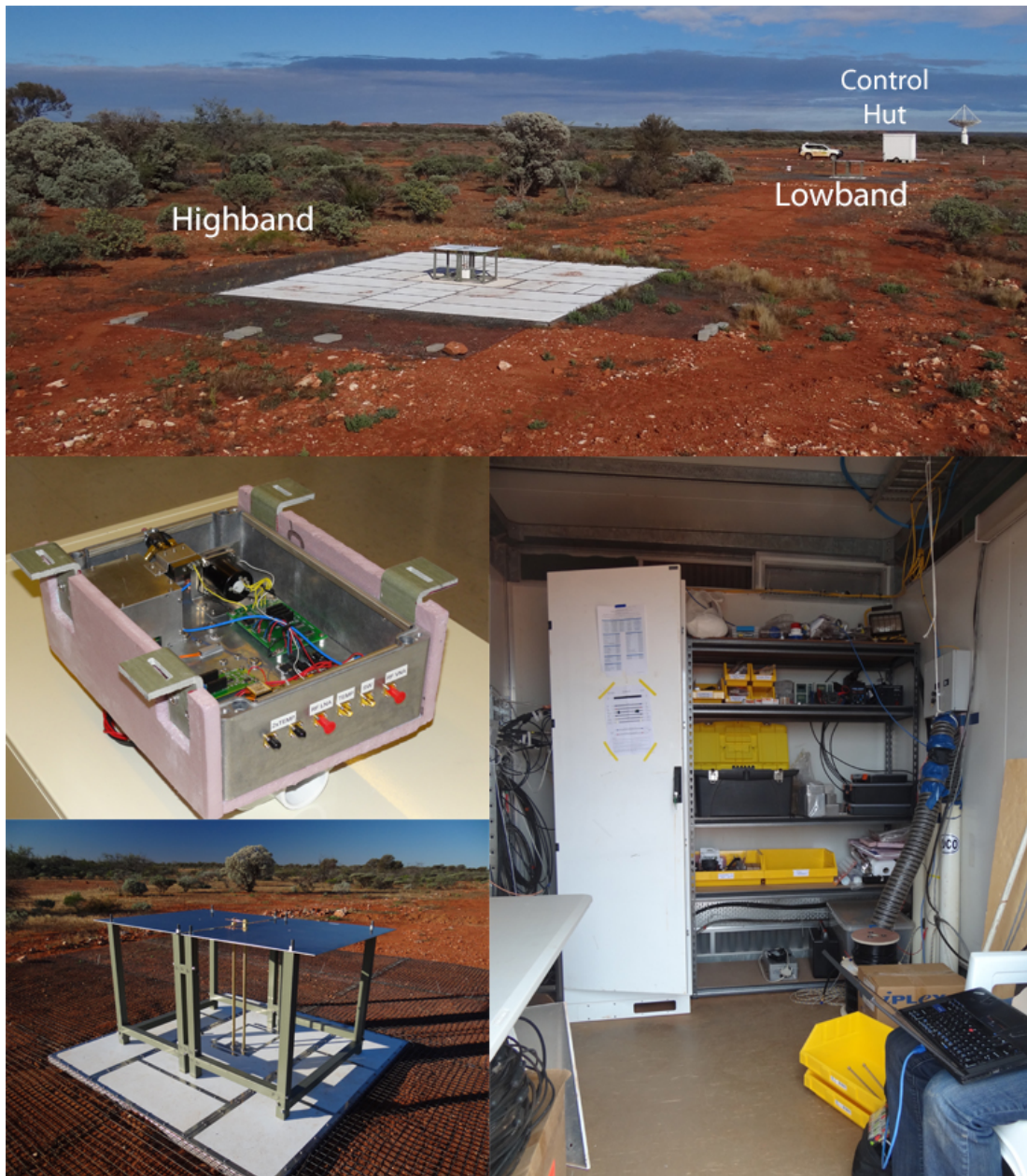
Figure 1.10: Blade highband and lowband systems July 2015 (see Table 1.1). The highband blade can be seen in the foreground along with the solid ground plane and the 2 x 5 m mesh extensions. The lower panels (clockwise from the right) show the inside of the control hut revealing the forced air conduit on the wall on the right in the back, the lowband antenna, and the inside of the highband receiver showing the pink insulating foam on the outside. Between the equipment hut and the highband is the lowband blade antenna. An ASKAP dish can be seen in the background behind the equipment hut.
