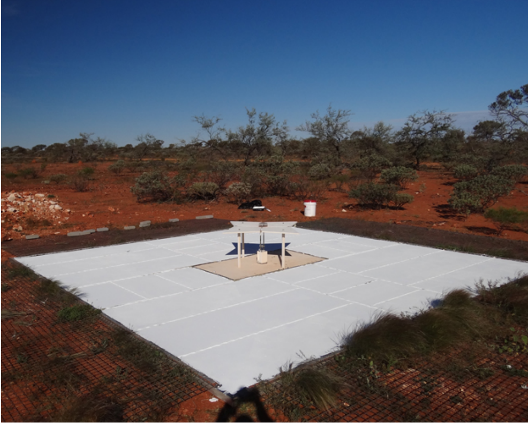
Figure 1.9: The fourpoint antenna (April 2015) would be replaced in July 2015 with the better performing blade antenna (see Table 1.1).
