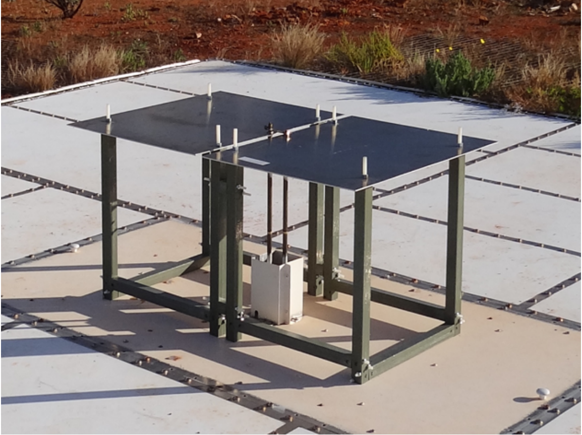
Figure 3.1: Photograph of the high-band blade antenna with fiberglass support tubes and a tuning capacitor on the top of the panels between the balun tubes to improve impedance matching. Surrounding the balun tubes at the base, a short rectangular enclosure shields against vertical currents in the tubes.
