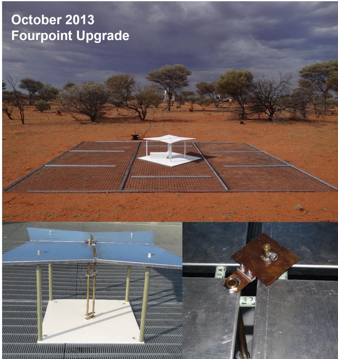
Figure 1.8: Intermediate upgrade to the EDGES instrument (see Table 1.1). The receiver enclosure can be seen on the central solid ground plane in the center photo. The solid ground plane sits atop a 5 m x 5 m mesh ground plane. The top capacitor is seen in the far right photo and the tuning capacitor is seen between the balun tubes in the left photo, which was taken atop the ISTB4 building at Arizona State University in Tempe, Az. during antenna characterization. Also seen in the left photo in the gaps between the panels at the edges are the quartz spacers used to control capacitance.
