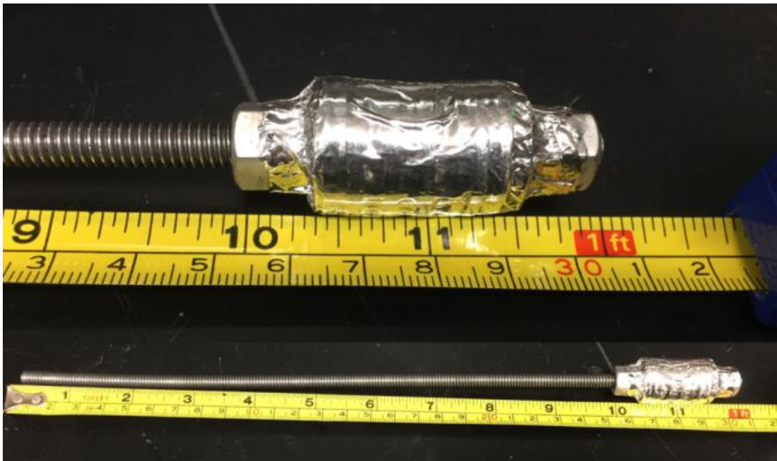
Figure 2.12. Magnetic Retrieval Tool. The magnetic retrieval tool used in this study was fabricated using aluminum hardware and most notably included a stack of 4 neodymium ring magnets (0.75”/0.375” outer/inner diameter) covered by aluminum tape.
