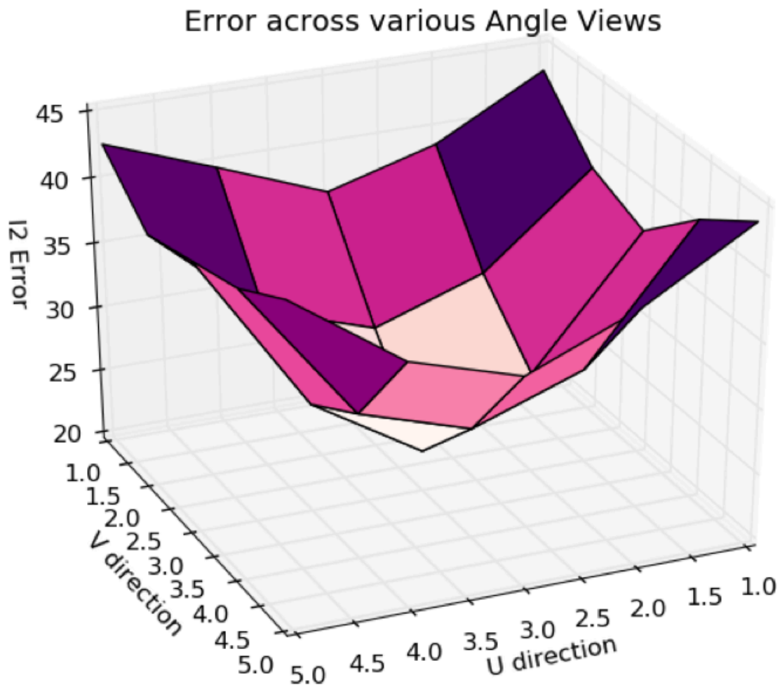
Figure 4.4: Error in Angular Viewpoints: Here we visualize the \ell_2 error for a light field reconstruction with respect to ground truth using a standard \ell_2 loss function for training. Notice how the extreme angular viewpoints contain the highest error. This helped motivate the use of a weighted \ell_2 function for training the network.
