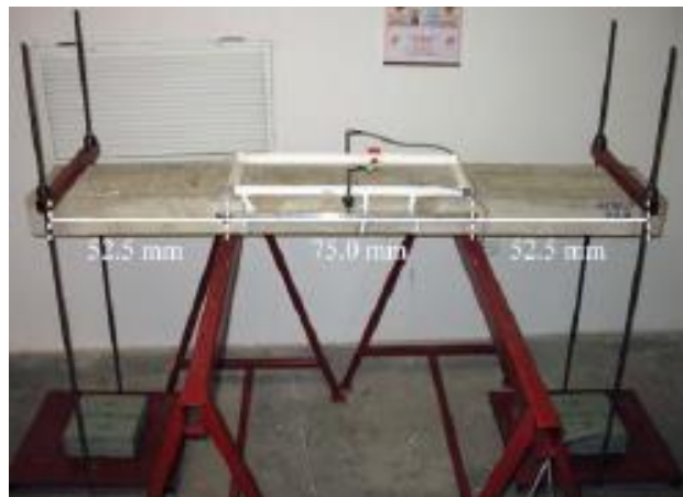
Figure 7: Creep Testing Set-up used by Buratti et al [Error! Bookmark not defined.]
