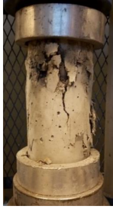
Figure 17: Concrete Cylinder after compression failure
