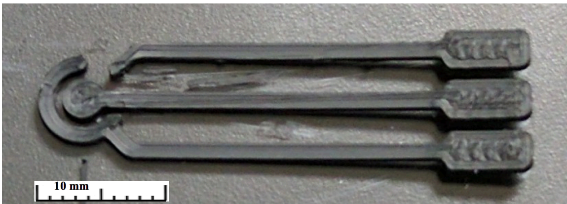
Figure 21: Gamma prototype of 3D-printed sensor made from conductive graphene filament onto a mylar substrate.
