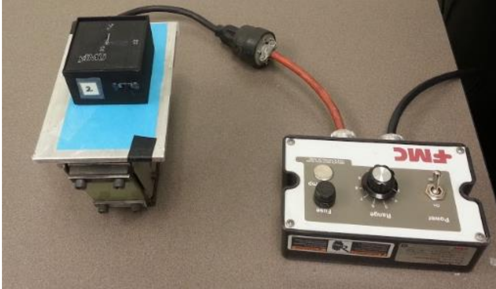
Figure 2.28: The FMC shaker used for vibration testing
