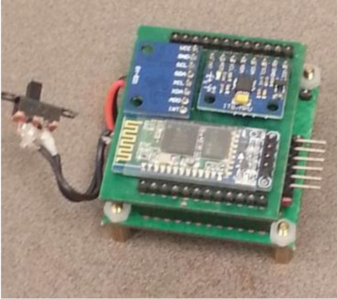
Figure 2.20: The stacked boards in yIMU v1.4
