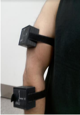
Figure 3.8: yIMU placement on subject body
