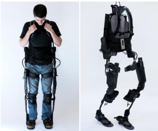
Figure 1.9: eLegs developed at Berkeley Robotics and Human Engineering Lab (eLegs 2010)
