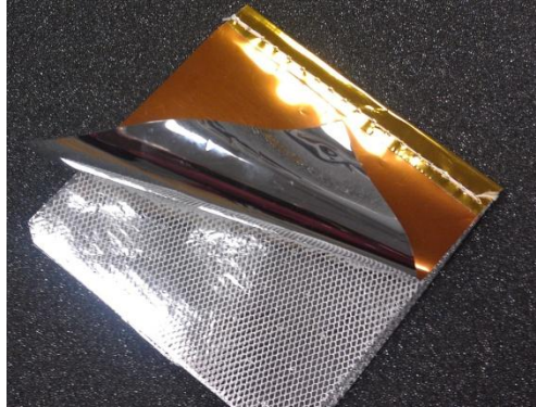
Figure 7-MLI with Aluminized Kapton coating [11].
