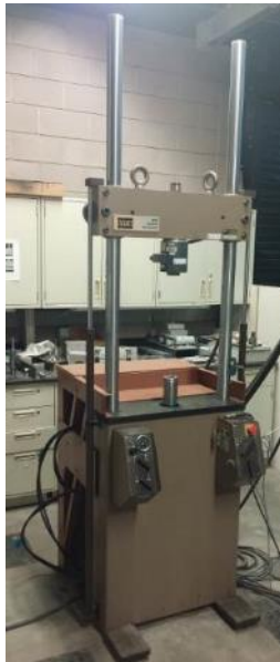
Figure 1. Photos of test equipment used in composites testing. MTS Load Frame (left) and Point Grey Grasshopper 3 camera set up (right)
