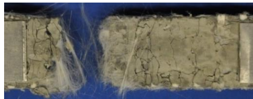
Figure 2-25 Representative Force-Strain Responses at Varying Temperatures for (a) GL-TRC, (b) SG-TRC, (c) PP-TRC and (d) Tested Specimens [46].
