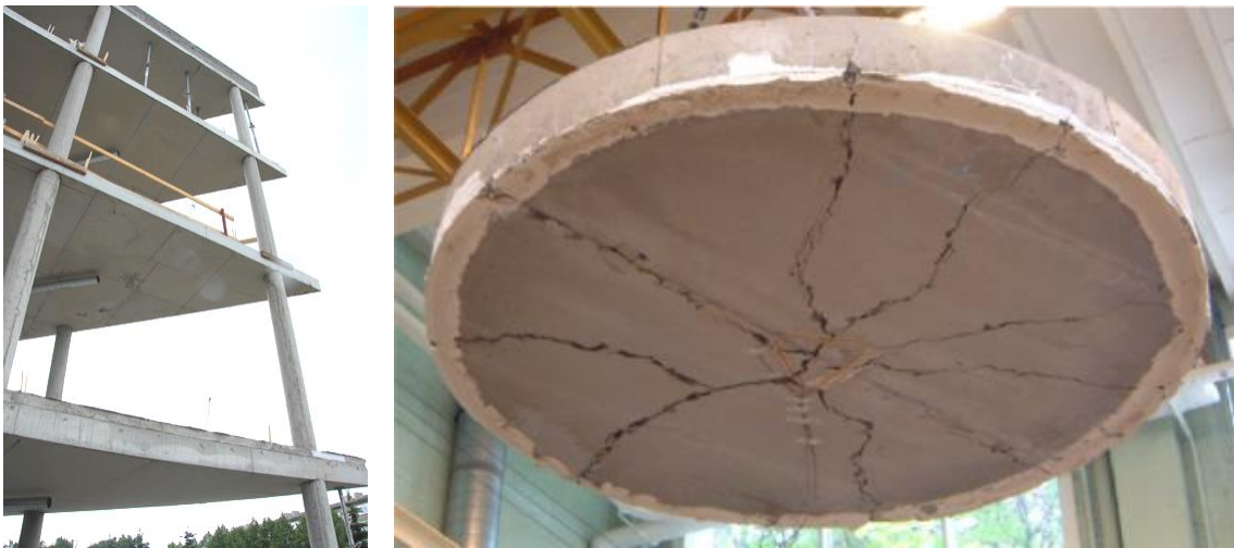
Figure 1-2 Construction and Applications of SFRC Slabs as the Main Reinforcing Material Used in Multistory Buildings. b) Failure Patterns of Distributed Fan Cracking Patterns in a Round Panel Test Method.
