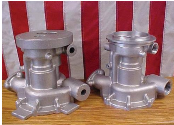
Figure 1: As Cast Part (L), Machined Part (R) [1]
