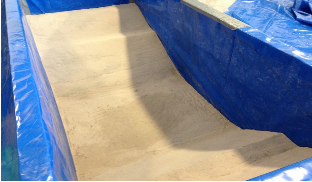
FIG. 4.2. Cemented sand landfill foundation within the centrifuge model container.
