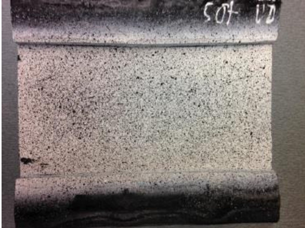
FIG 5.4. HDPE coupon prepared with speckle pattern.
