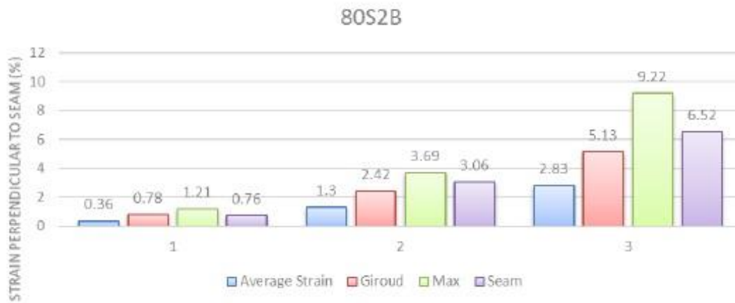
FIG 5.16. 80-mil dual hot wedge seam strains (80S2B).
