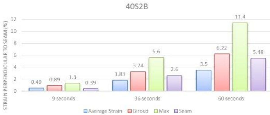
FIG 5.13. 40-mil dual hot wedge seam strains (40S2B).
