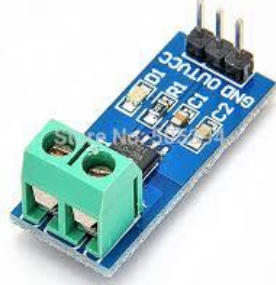
Figure 49 - ACS712 Current Sensor an analog signal and is connected to the Arduino.
