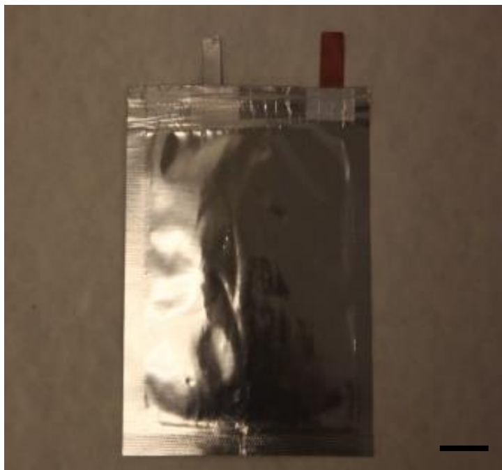
Figure 2.3. Optical image of an assembled LIB. Scale bar is 2 cm.
