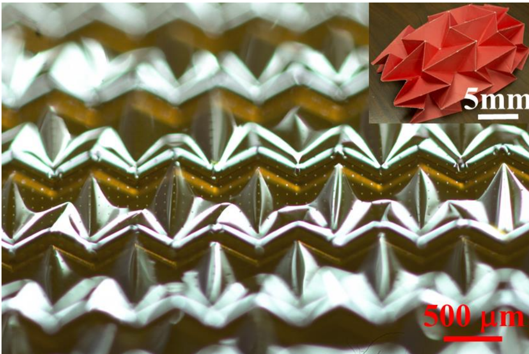
Figure 4.8. A photography of a Si NM ‘magic ball’ pattern. The inset shows a paper-based Miura-ori pattern for comparison.
