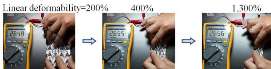
Figure 2.9. Photograph of linear deformation (i.e., folding and unfolding) of an origami LIB while it was connected to a voltmeter.
