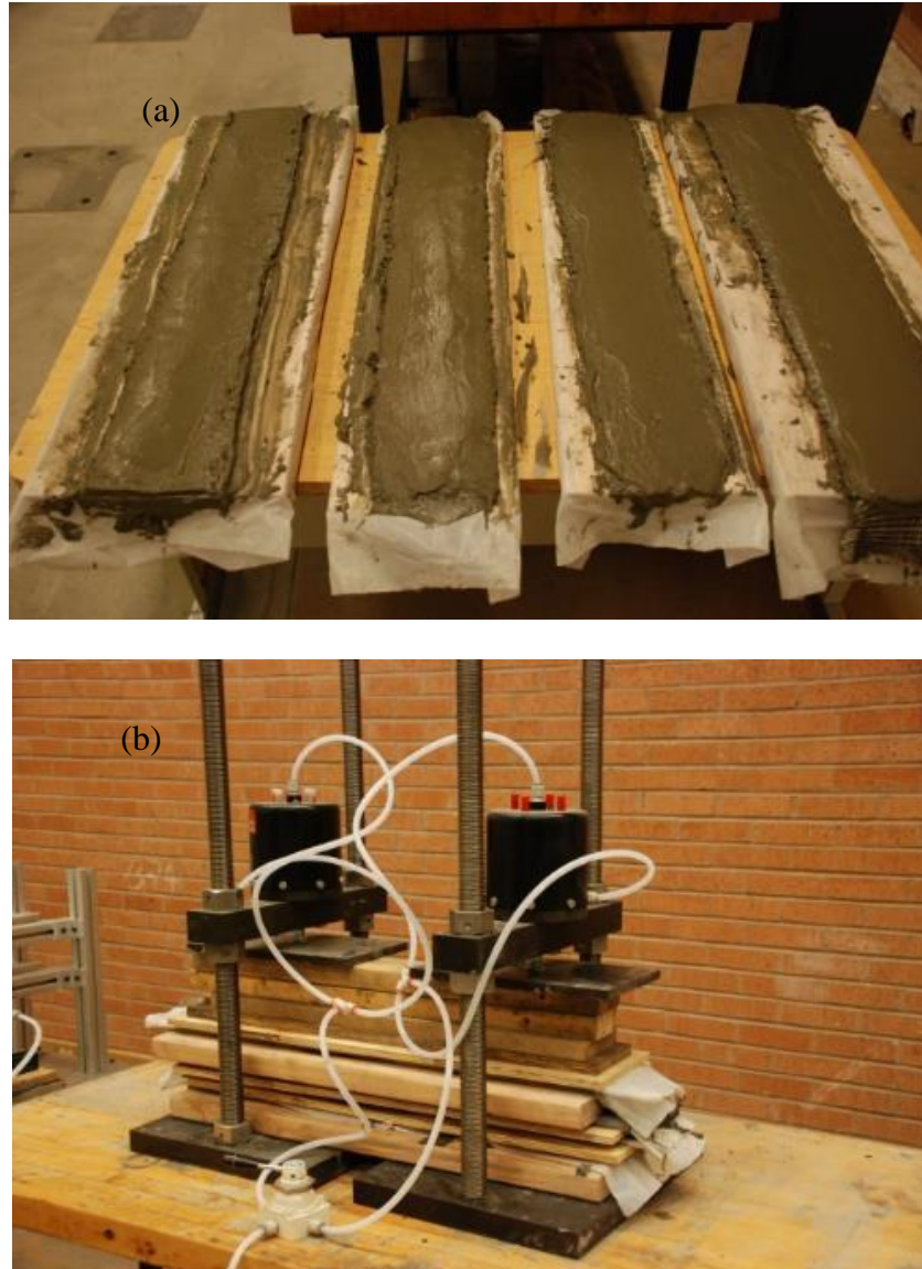
Figure 3-11: (a) Multiple plate samples cast in one session; (b) Pressing of multiple plates
