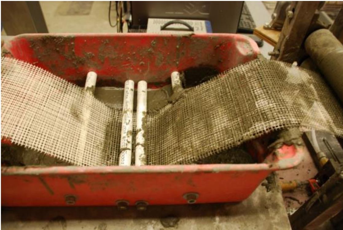
Figure 3-3: Textile passing through paste bath
