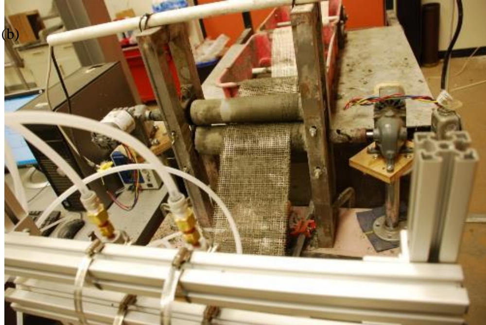
Figure 3-4: (a) Textile being pulled through the treatment baths, (b) pultruded textile squeezed in between the rollers powered by DC motors
