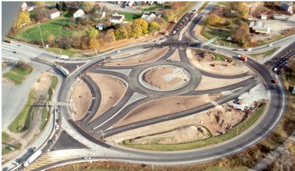
Figure 2: Small modern roundabout vs. large traditional rotary or traffic circle.
