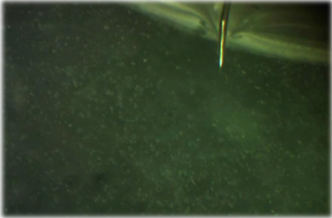
Figure 23 A frame after the initial penetration of electrode inside the PDMS.
