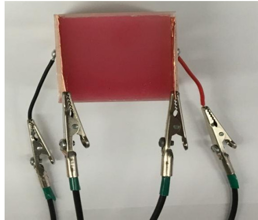
Figure 25: Pictorial representation of the measurement of impedance in high conductivity TX-151 gel in a sample chamber (5 cm x 5 cm x 5 cm) using four-probe electrode method.
