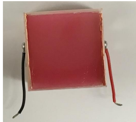
Figure 25: Pictorial representation of the measurement of impedance in high conductivity TX-151 gel in a sample chamber (5 cm x 5 cm x 5 cm) using four-probe electrode method.
