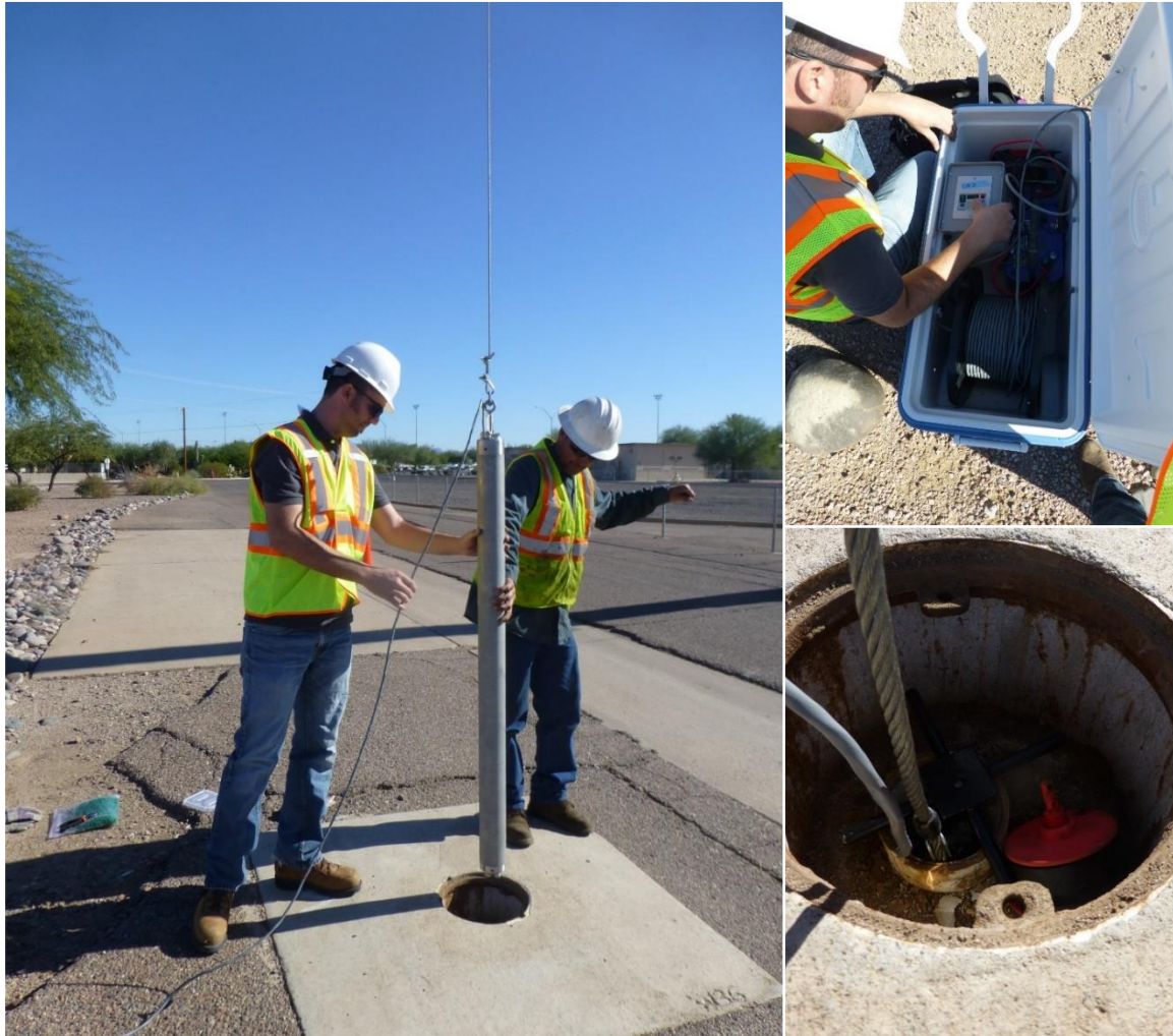
Figure E.4: Deployment of the IS2 sampler into W36 at the former Williams AFB, November 2013. Clockwise from left: 1) insertion of the sampler by crane, 2) the surface package being programmed, and 3) the deployment hanger on the well head (Photographs by Sara Murch).
