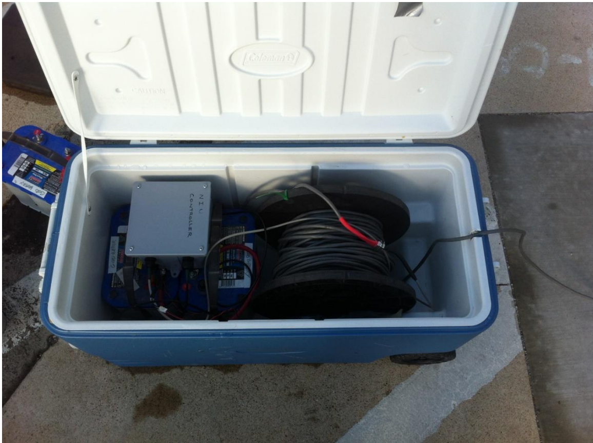
Figure C.2. Surface package providing power and communication channels to the submersible sampler. A weather-tight case houses a 24-V battery pack, a USB interface for communication, and spool of 9-channel cable driving the submersible unit (Photograph by the author).
