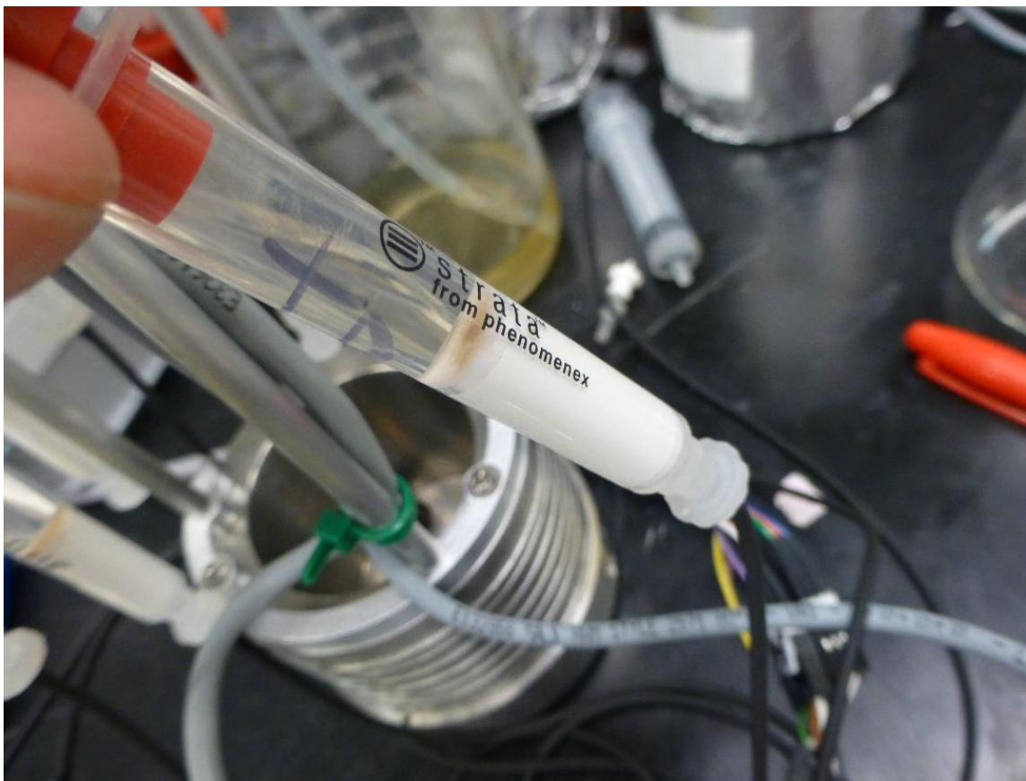
Figure D.3. Accumulation of surface water sediments upon the frit of an SPE cartridge (Photograph by Samuel Supowit).
