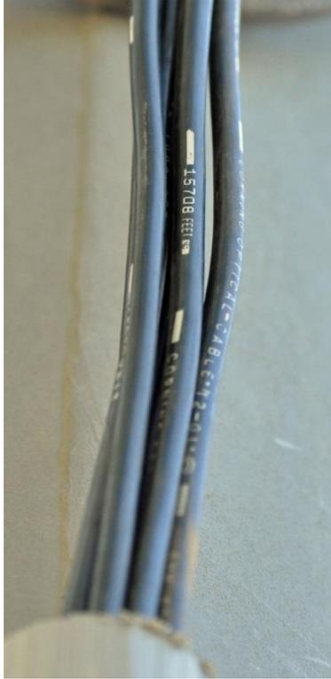
Figure 6.4: Length Markings on Corning Fibers
