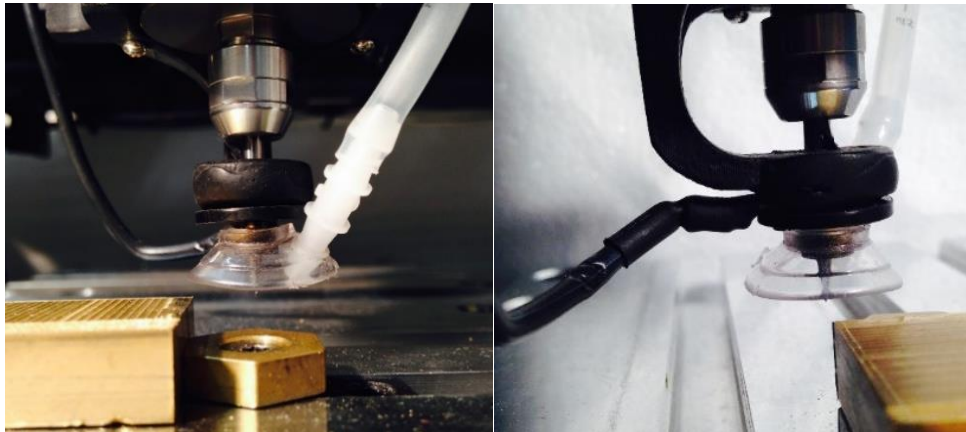
Figure 15: (L to R): Front view and side view of the skirt and suction tube
