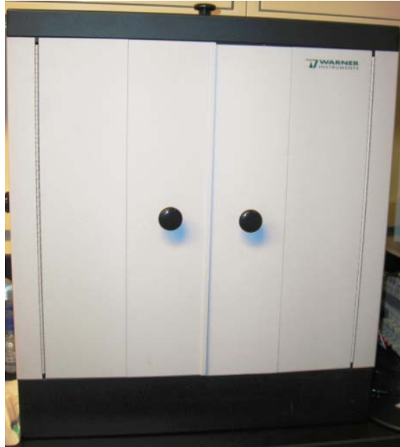
Figure 3. 9: Faraday cage for electric noise and mechanical vibration isolation.
