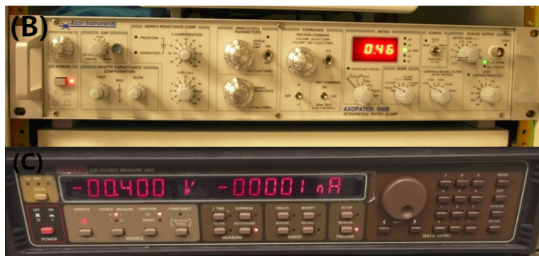
Figure 3. 6: Electrical setups. (A) Electrical set up illustration for the nanopore aqueous ionic current measurement with chip bias modulation. (B) Picture of Axopatch 200B Low Noise Current Amplifier. The red number shows the noise level. (C) Picture of Keithley 236 source measure unit. The left number shows the DC Voltage applied and the right current number shows the current received from the wire.
