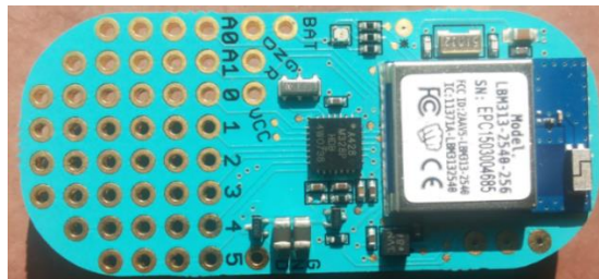
Figure 8. Lightblue bean: Processing Unit of Smart Glove
