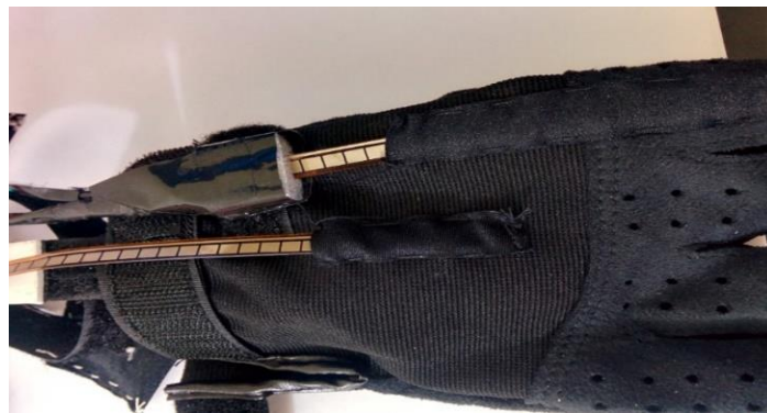
Figure 10. Resistive Strip Sensors Mounted on the Glove Using Stitched Pockets
