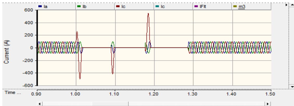
Figure 3.17: Recloser Operation in Mode 2
