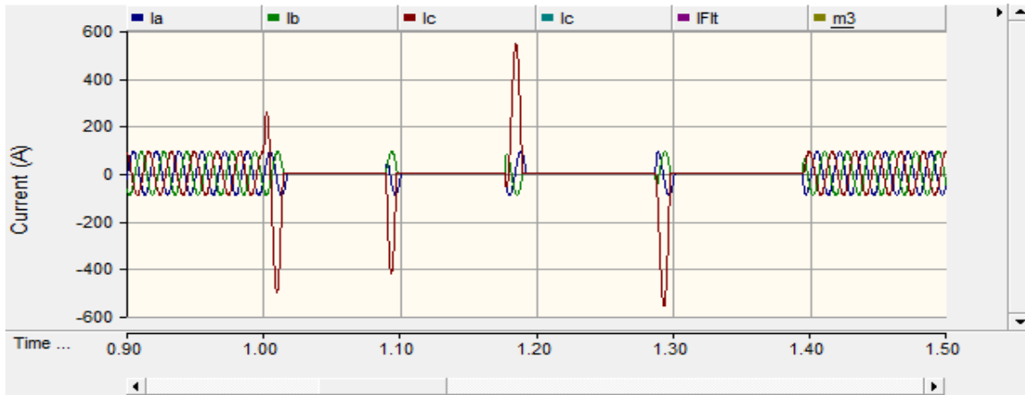
Figure 3.18: Recloser Operation in Mode 3
