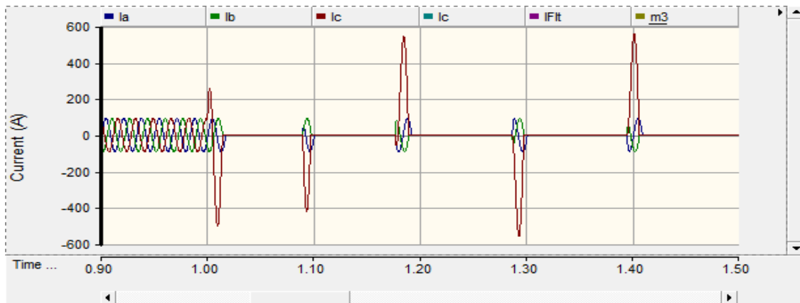
Figure 3.19: Recloser Operation in Mode 4
