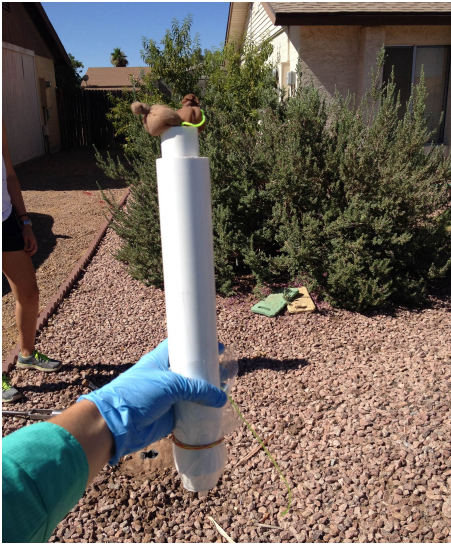
Figure A1. The 30cm depth resins were installed using a double-PVC pipe apparatus. The outside larger pipe was permanently installed at an angle in the soil during the study. The smaller, inner pipe, was used to hold and replace the resins. The resins sat at the bottom end of the tube (shown here upside down) and the opposite end was capped using plastic sheeting to prevent any precipitation or irrigation water reaching the resin bags that did not first travel through the soil column.
