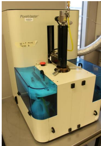
Figure 3-2: Quantachrome PoreMaster mercury intrusion porosimeter
