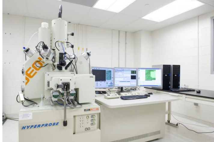
Figure 3-6: JEOL JXA-8530F Hyperprobe featuring Field Emission Scanning Electron Microscope (FESEM) surrounded by five Wavelength Dispersive Spectrometers (WDS)
