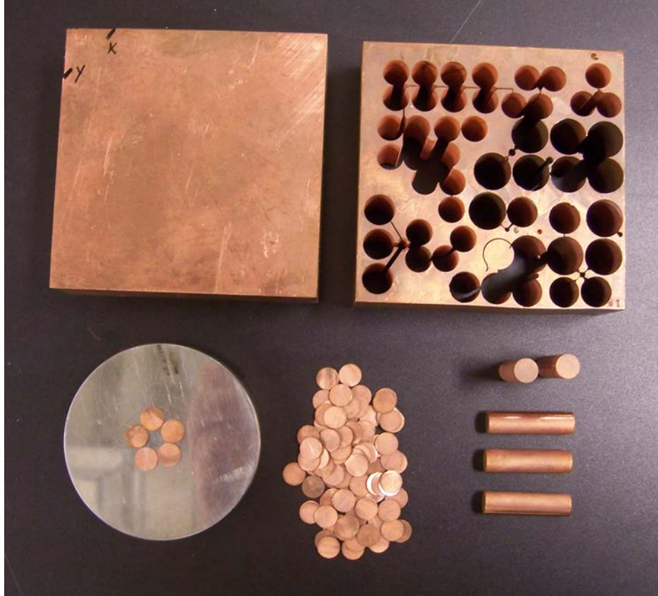
Figure 13: Clockwise from top left: raw plate of half-hard copper, EDM manufacturing of cylinders of appropriate diameters for flyers and targets from raw material, bored out cylinders, EDM discs from bored cylinders, discs awaiting polishing on a sample holder that fits onto the polishing machine.
