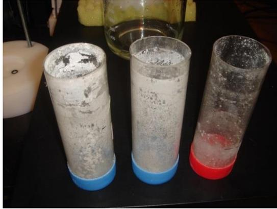
**Figure 16** Percolation Acrylic Columns #1, #2, #3 (left to right). Acrylic Columns #1 and #2 showing carbonate mineral precipitate along the inside walls.
