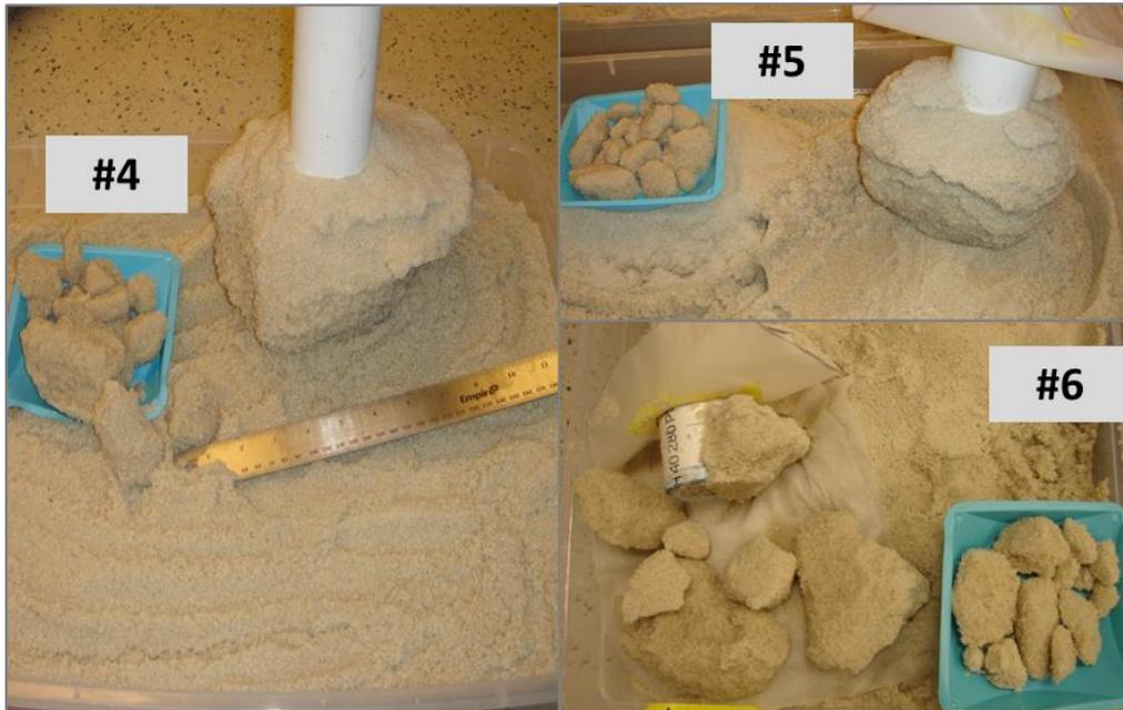
**Figure 31** Bulb-shaped cemented soil masses from wet Buckets #4-6. Note that the apron in Bucket #6 moved down the injection tube during pullout.
