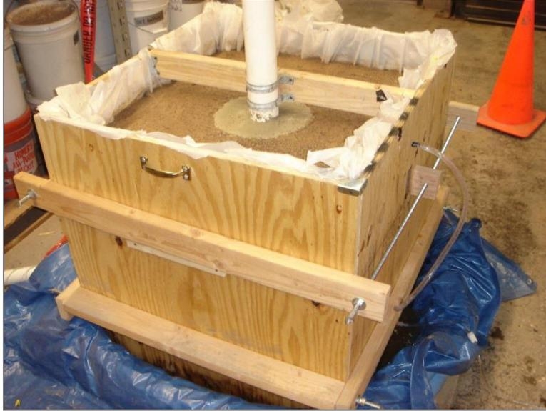
**Figure 27** Soil-filled box with Na-bentonite seal around injection tube.
