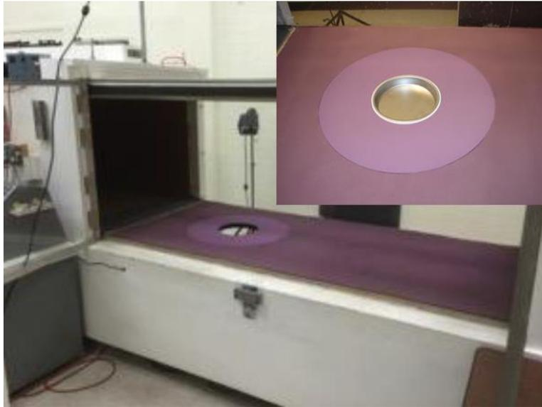
**Figure 37** Wind tunnel stage area. The inset photograph shows the arrangement of the adapter ring (white) and cake pan in the wind tunnel.
