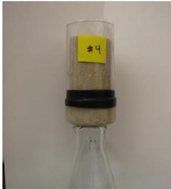
**Figure 13** Sand-filled acrylic column before adding the EICP reaction medium.
