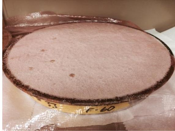
**Figure 38** Treated soil pan containing F-60 silica sand loosely covered in plastic wrap.
