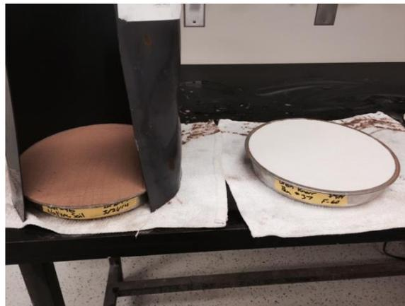
**Figure 36** Two soil pans native sand (left) and F-60 sand (right) prior to treatment. Black PVC shield was used to reduce overspray.
