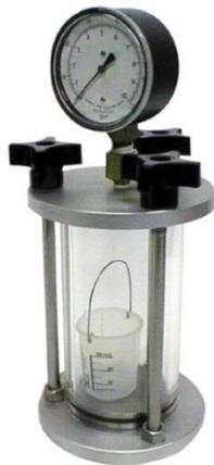
**Figure 1** Apparatus for measuring CO<sub>2</sub> production via acid digestion of CO<sub>3</sub><sup>2-</sup> minerals.
