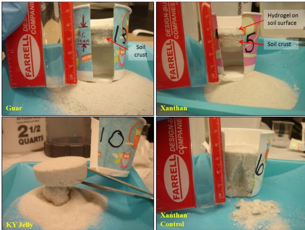
**Figure 43** Paper cups were cut open longitudinally to provide a “window” view of the soil profile. The cups were tilted and tapped to allow loose soil to pour out.
