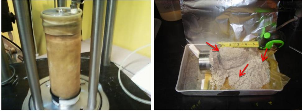
**Figure 21** Triaxial sand Column #1 standing without support with a weighted stainless steel top-cap (left image). A large strongly cemented center and several broken pieces found after triaxial testing (right).
