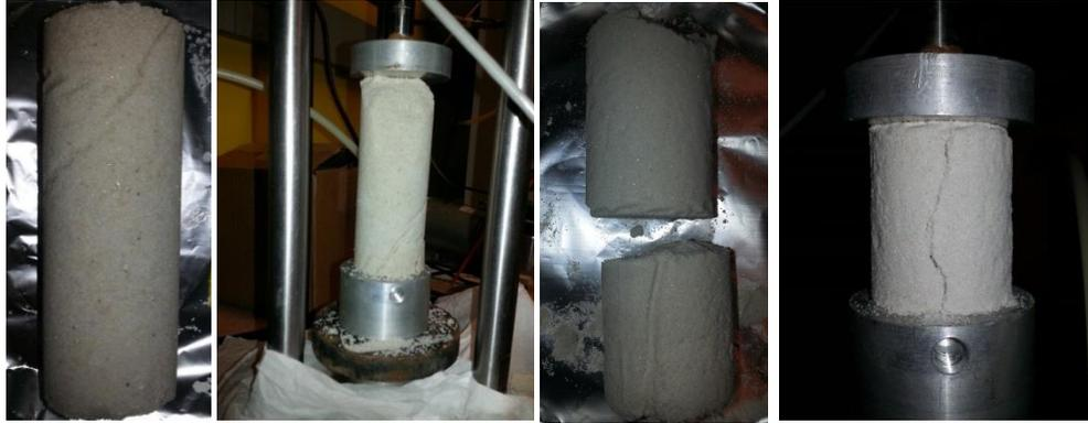
**Figure 23** Acrylic Columns #4-5 prior to and during UCS testing. The 2 left images are 20-30 sand and the 2 right images are F-60 sand.
