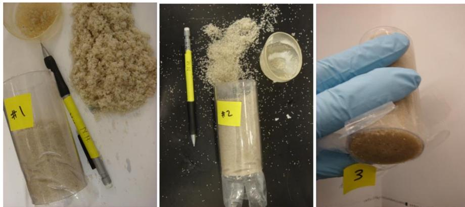
**Figure 14** Columns #1-2 (0.20 M) and #4 (0.5 M) before extraction. Soil exposure due to evaporation was most notable in Column #1.
