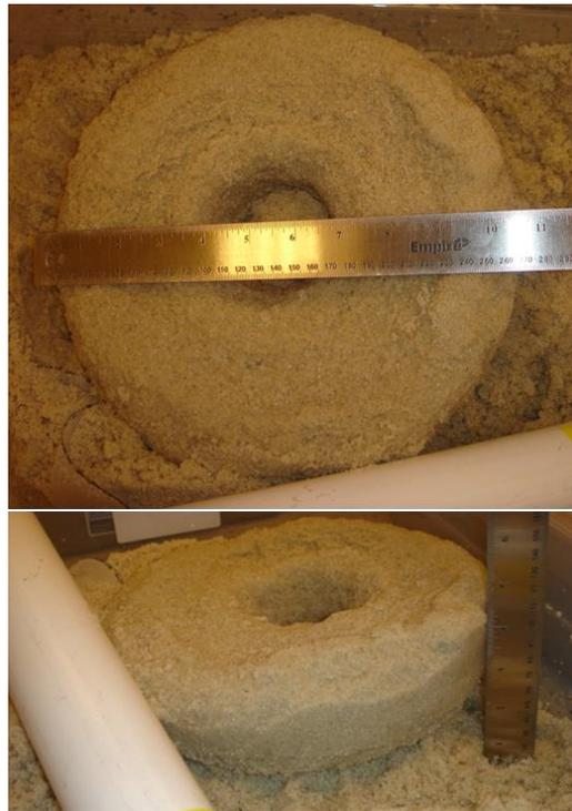
**Figure 30** Donut-shaped cemented soil mass from dry Bucket #2.
