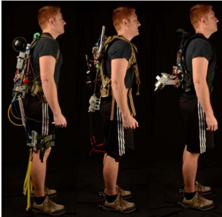
Figure 1.8. Devices Designed to Augment Human Running. From Left to Right, AirLegs V1, AirLegs V2, and Jet Pack
