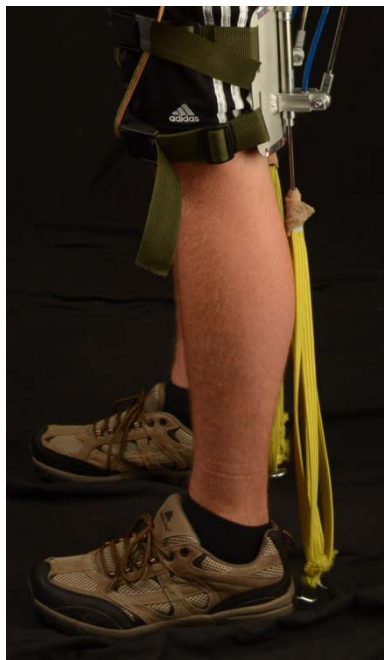
Figure 4.3. Actuator Assembly Connected to Heel to Provide Torque at the Ankle
