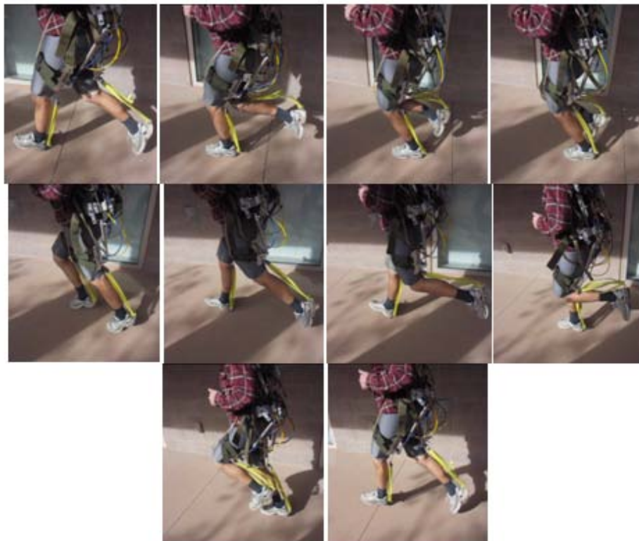
FIGURE4.4. AirLegs V1 Gait Cycle; from left to right, top to bottom, the device pulls the left leg back during the stance phase and applies torque at the ankle during push off. The device then pushes the leg forward during the swing phase.
