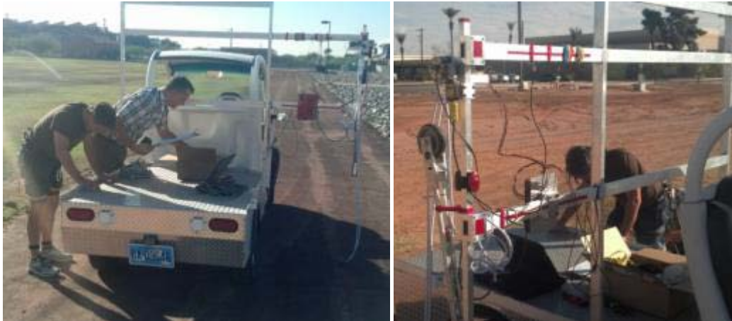
Figure 2.5. Testing Rig Attached to an Electric Golf Cart
