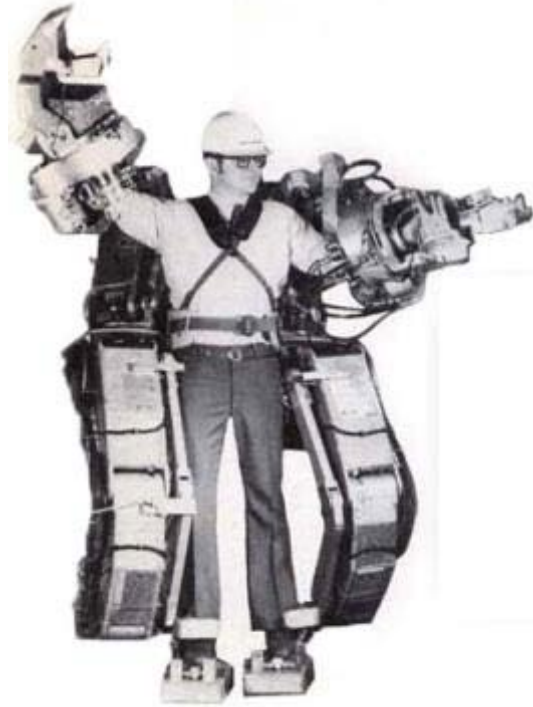
Figure 1.6. Hardiman Designed by General Electric (General Electric, 1968)
