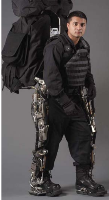
Figure 1.7. BLEEX Exoskeleton Designed by Berkeley Researchers (Chu, 2005)
