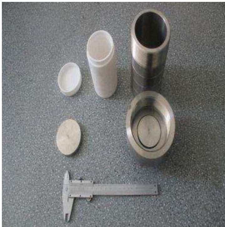
Figure 1.3.1 Teflon-lined stainless steel reactor usually used in hydrothermal/solvothermal synthesis of MOFs.
