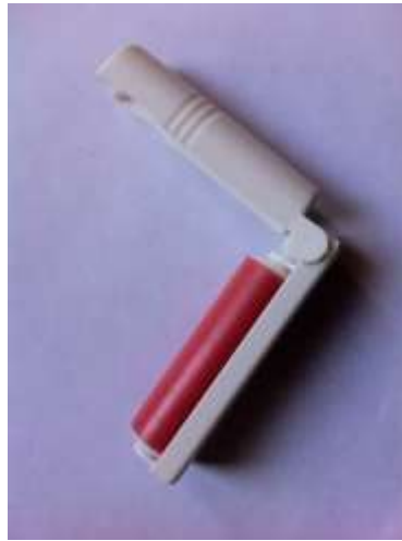
Figure 8.3 Mini washable lint rollers used for dust sampling
