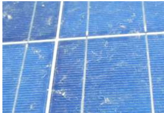
Figure 9.5 Soiling in Goodyear, AZ (Tilted 22°, ET=76 days)
