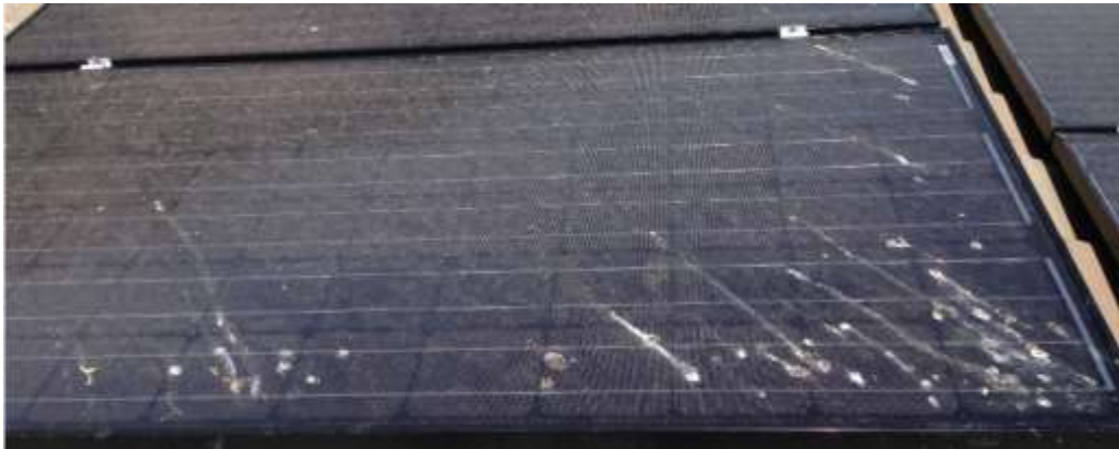
Figure 9.4 Heavy bird droppings found in Mesa, AZ (Tilted 17°, Exposure Time (ET) =82 days)
